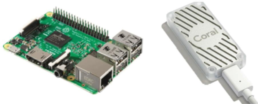
**Figure 7.** On the (left), we have the general-purpose embedded platform, represented by the RPi 4 B, while on the (right), we have the TPU-based platform, represented by the USB Coral TPU.
