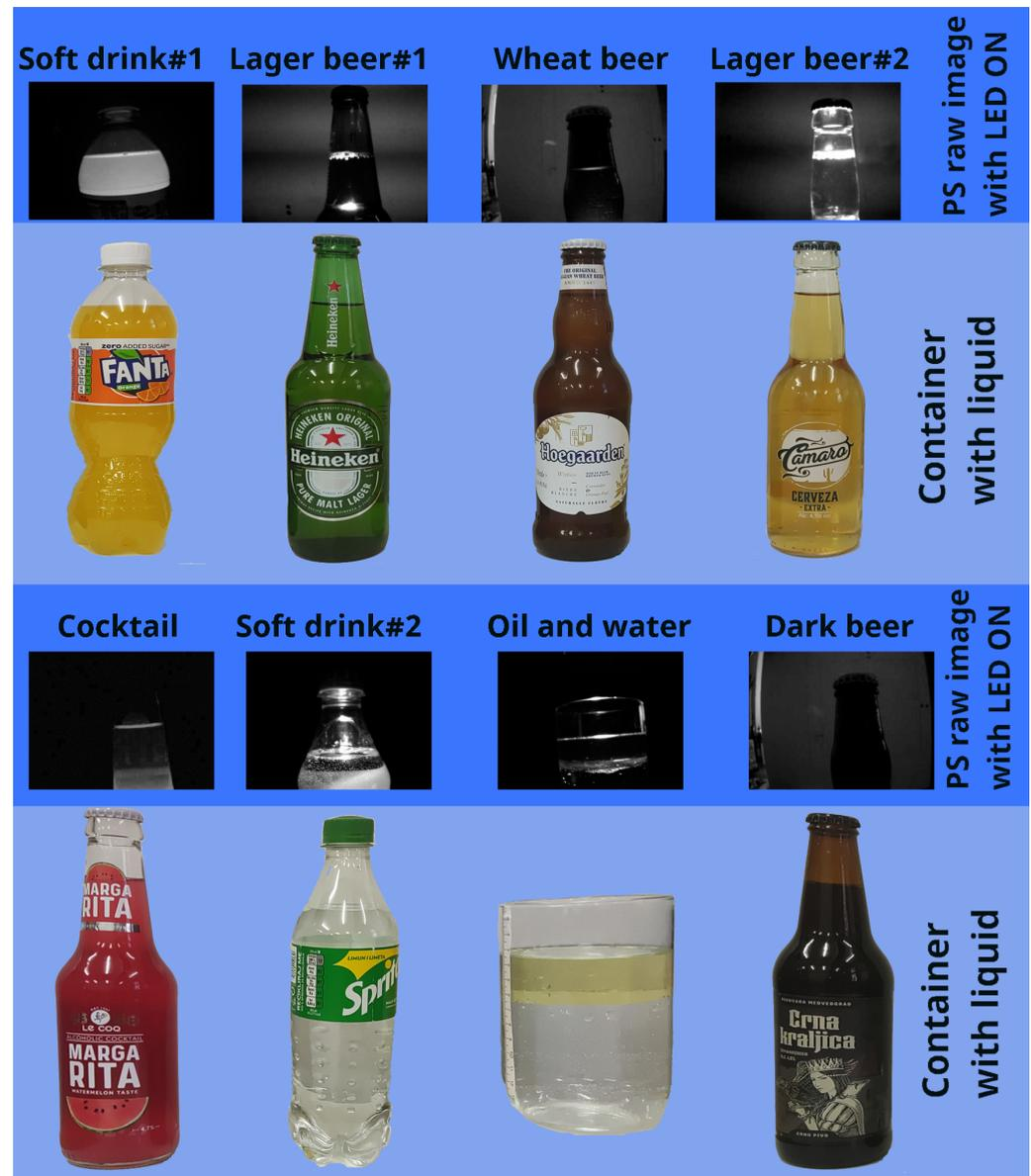
**Figure 19.** The light pattern required for the successful operation of the PS, observed during the measurement with different bottle shapes and liquids (obtained using OptoSupply OSW4XAHA1E, a 10 W cool white 850 lm LED source).
