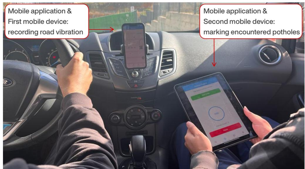
**Figure 3.** Data acquisition process in the vehicle using smartphone sensors and mobile application.
