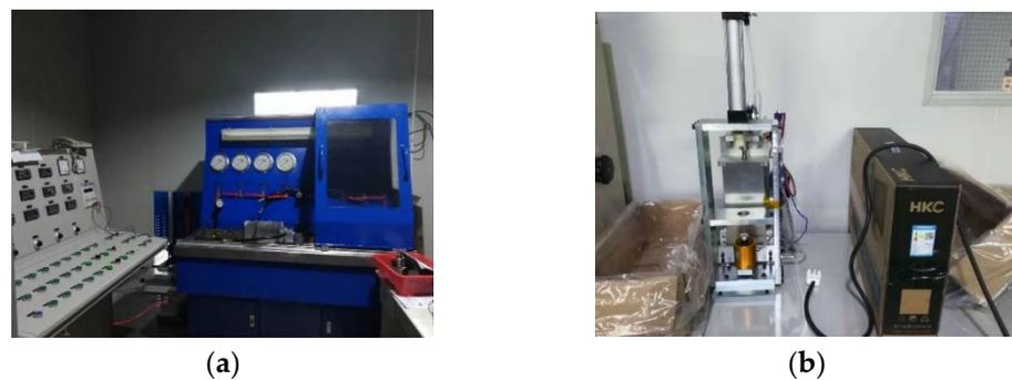
**Figure 6.** Independent test equipment of proportional solenoid valve in non-installed state. (a) Hydraulic pressure test platform; (b) Electromagnetic force test platform.
