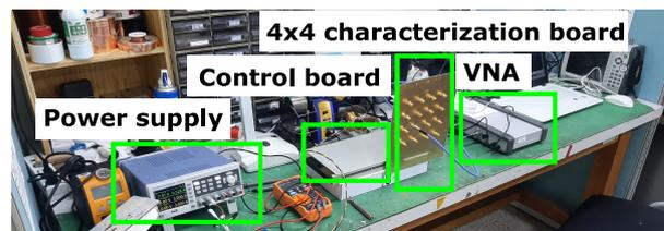
**Figure 10.** Measurement setup for determining the phase shift profile.
