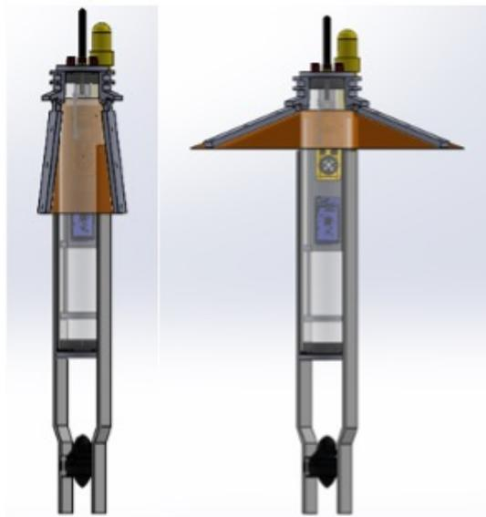
**Figure 1.** A model of the considered floater. In the left panel, the floater's arms are close, while in the right one, they are open.
