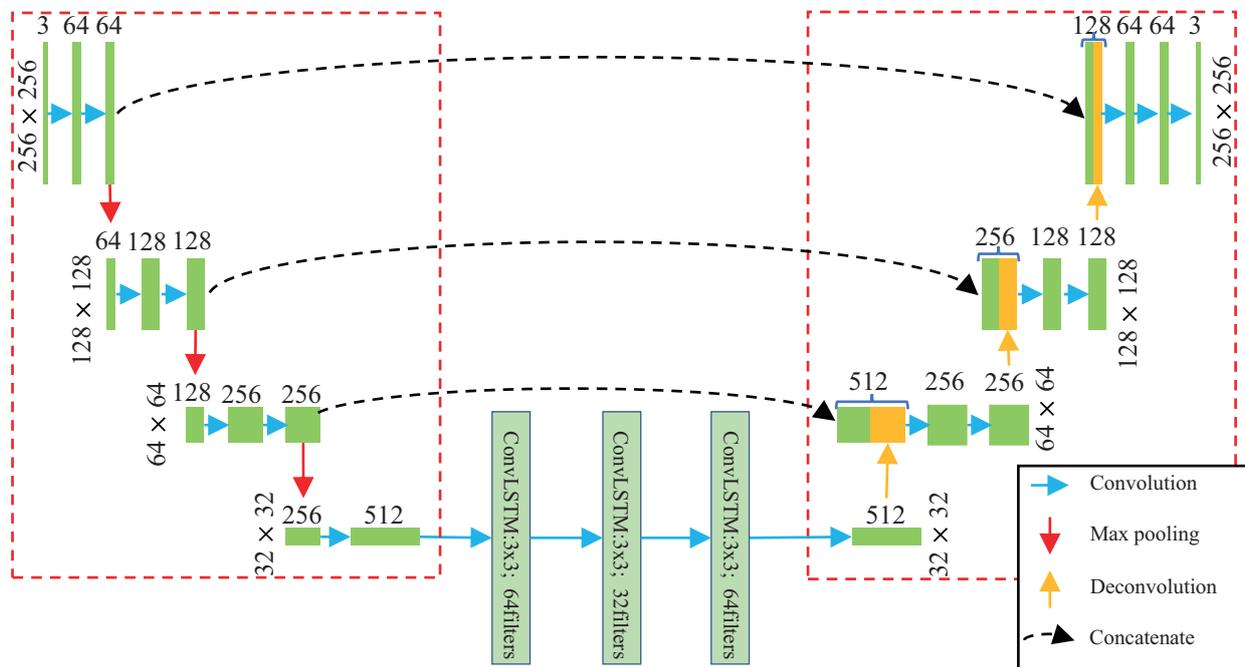
**Figure 3.** The detail of the network structure of our work. There are three zones in the network, in which the left zone is called the encoder, the right zone is called the decoder, and the rest of the structure in the middle is the LSTM network.
