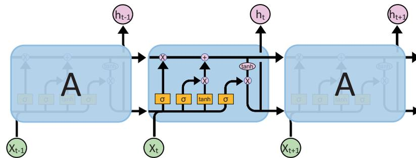
Figure 2. LSTM structure.
