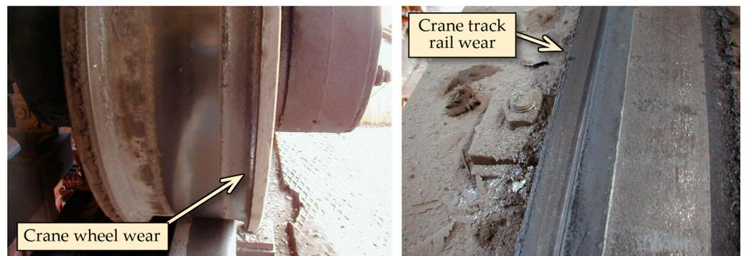
**Figure 3.** Examples of wear on the crane wheels and crane track rails.
