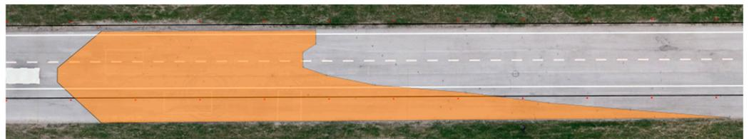
**Figure 29.** C 9.5 class road (I, II, III)—ankle-height illumination—Hyundai i40.
