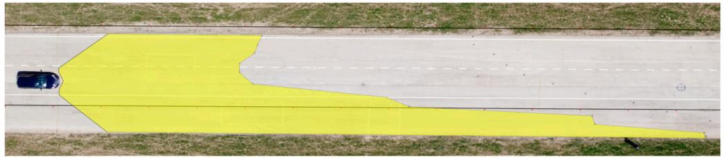
Figure 20. C 9.5 (I, II, III) class road—knee-height illumination—Dacia Sandero.
