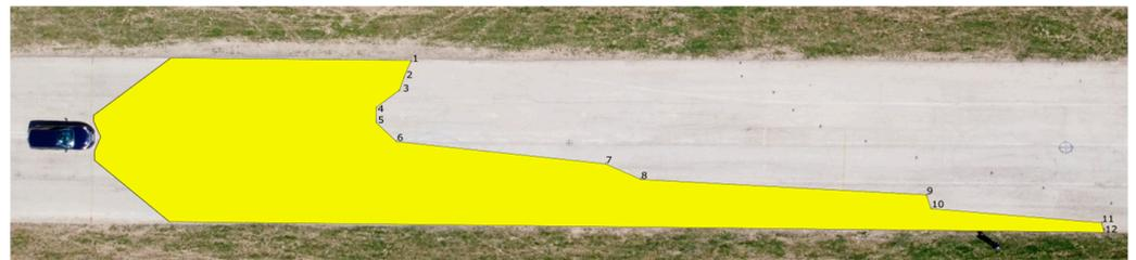
**Figure 9.** Range of visibility at knee height—Dacia Sandero.
