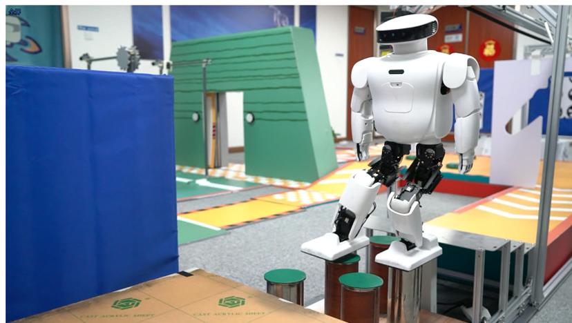
**Figure 11.** Discrete terrain walking. The walking area is limited to two rows of support columns.
