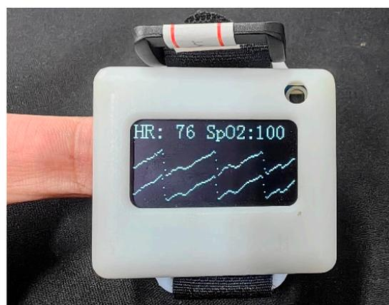
**Figure 2.** PPG data acquisition device.
