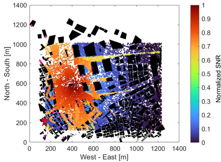
Figure 10. UE received SNR when using IRS & neighboring BS.
