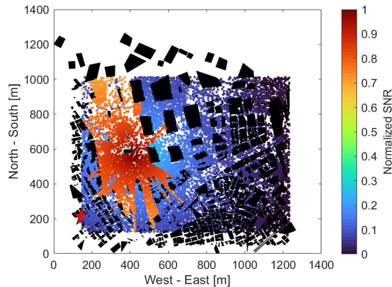
Figure 8. UE received SNR when not using IRS.
