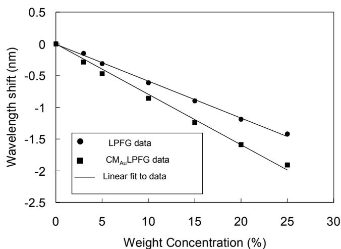
**Figure 14.** Wavelength shift of a bare LPFG sensor (black squares) and a CM<sub>Au</sub>LPFG sensor (black circles) in sodium chloride aqueous solution with increasing weight concentration.
