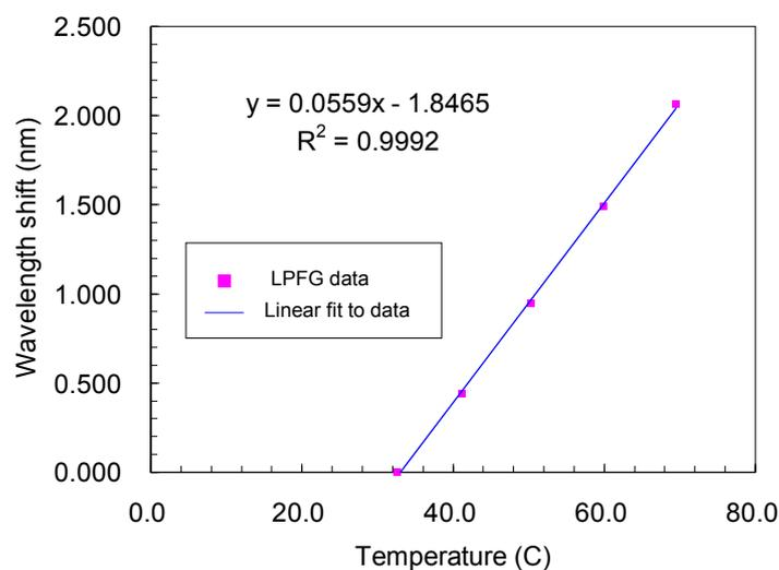
**Figure 6.** Wavelength shifts of a typical LPFG against temperature changes.
