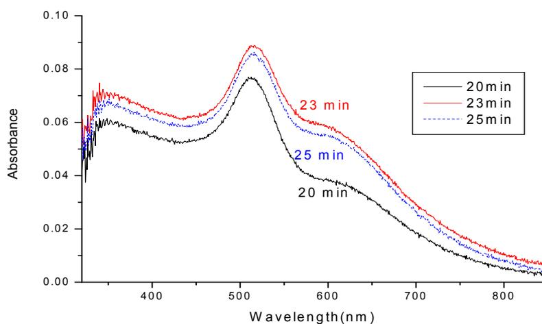
**Figure 5.** Absorption spectrum of  $CM_{Au}$ 's on glass substrate with three different self-assembled time.
