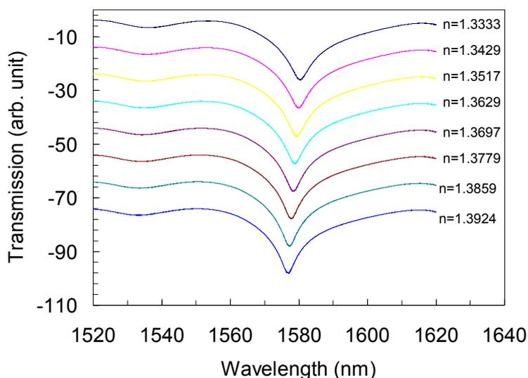
**Figure 11.** Transmission spectra of a typical LPFG in sucrose aqueous solution with increasing weight concentration.
