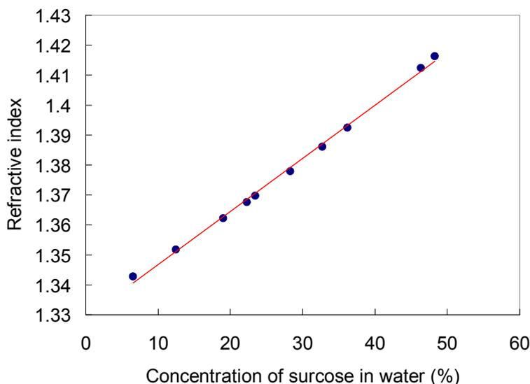
**Figure 10.** A plot of solution refractive index versus concentration of sucrose in the solution.
