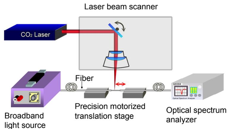
**Figure 3.** Schematic of experimental set-up for LPFG fabrication using CO<sub>2</sub> laser pulses.
