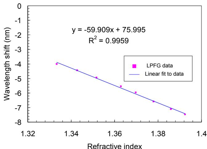
**Figure 12.** Wavelength shift of a bare LPFG sensor with increasing concentration of sucrose in aqueous solution.
