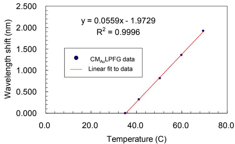
**Figure 7.** Wavelength shifts of the CM<sub>Au</sub>LPFG versus temperature.
