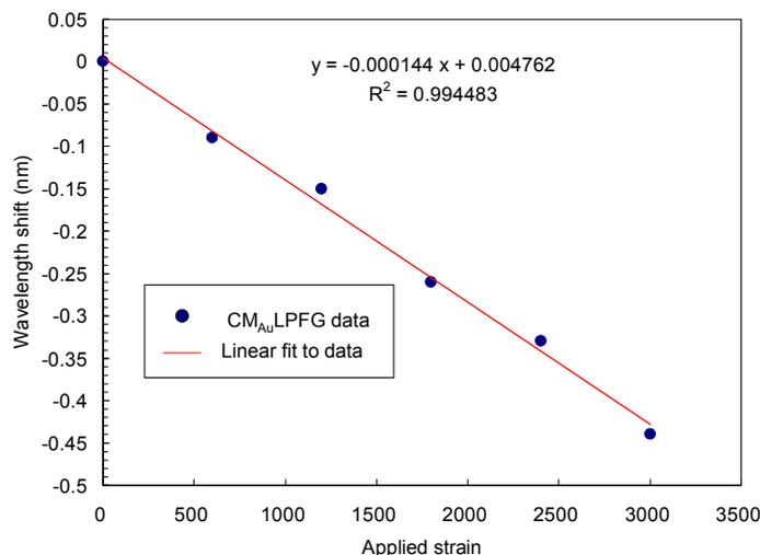
**Figure 9.** Wavelength shifts of the  $CM_{Au}$ LPFG versus strain.
