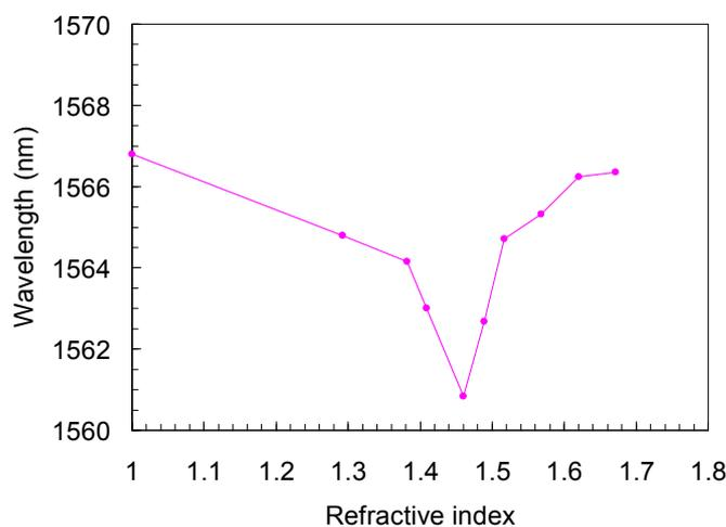
**Figure 2.** Wavelength shifts in one of the resonance bands of an LPFG with refractive index changes.
