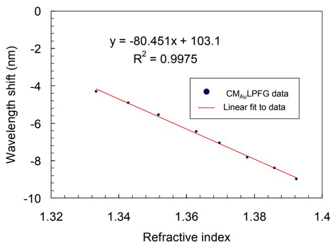
**Figure 13.** Wavelength shift of a CM<sub>Au</sub>LPFG sensor with increasing concentration of sucrose in aqueous solution.
