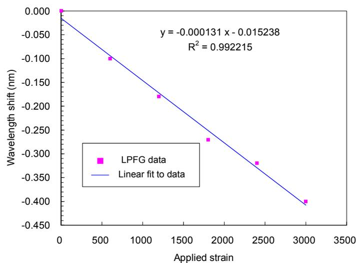
**Figure 8.** Wavelength shifts of the LPFG versus strain.
