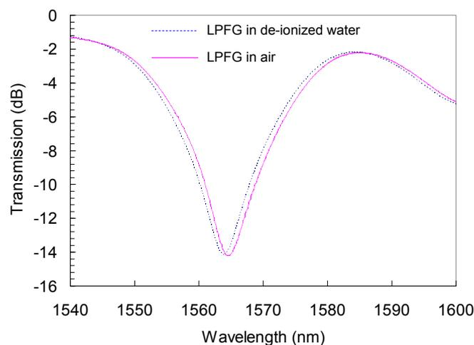
**Figure 1.** Transmission spectrum of an LPFG in air (solid line) and in de-ionized water (dash line).
