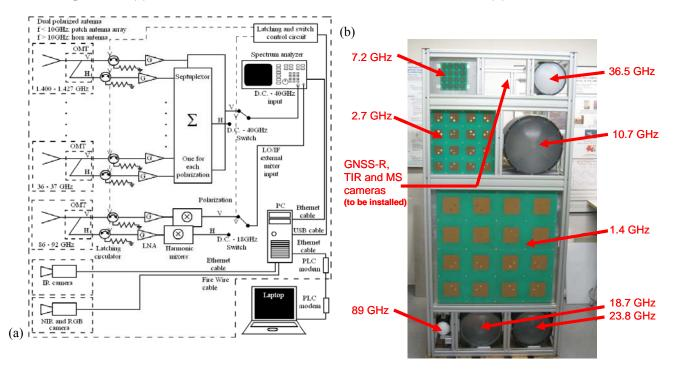
Figure 12. (a) MERITXELL microwave radiometer schematic, and (b) front view.
