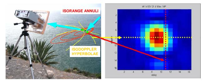
**Figure 4.** Measured (not normalized) 1 s incoherently integrated DDM with the threshold applied to compute its volume. Noise is well below the threshold [9].
