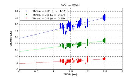
Figure 15. DDM-volume dependence on the SWH for three different thresholds [8].
