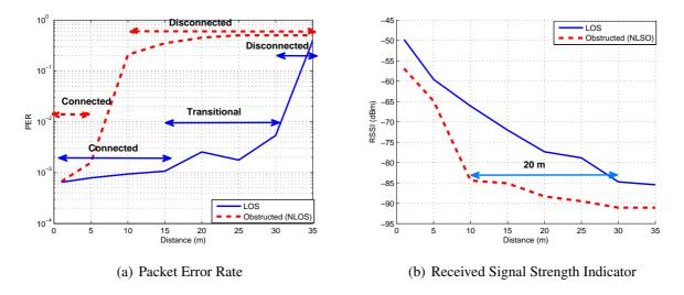
Figure 10. Distance region where two-hop PER is below  $5 \times 10^{-2}$ . Corridor Scenario.
