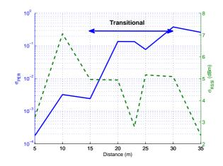
Figure 4. Standard deviation for PER and RSSI. Corridor Scenario.
