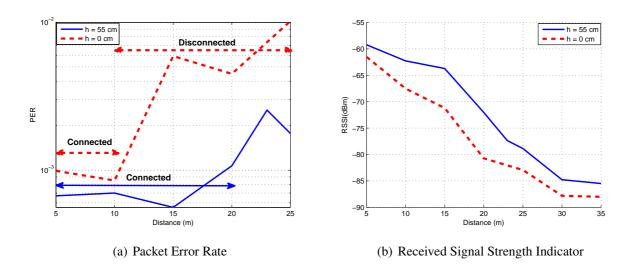
Figure 6. PER and RSSI against distance for two mote heights. Office Scenario.
