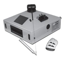
The Proliner has a cable with a length of 5 meters, so the maximum distance that can be measured with the Proliner from a station position is 10 meters (in absence of obstacles). The technical specifications of Proliner, according to the manufacturer, are the following:
