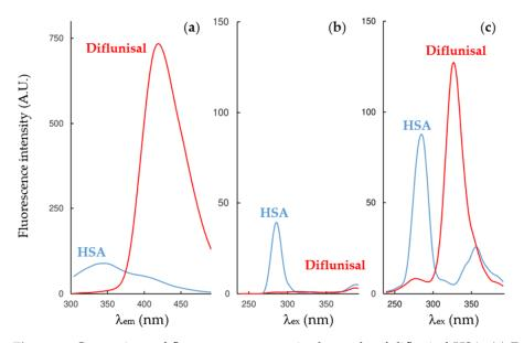
**Figure 1.** Comparison of fluorescence spectra in the study of diflunisal-HSA: (a) Emission; (b) synchronous  $\Delta\lambda$  15 nm; (c) synchronous  $\Delta\lambda$  60 nm modes at 25 °C.
