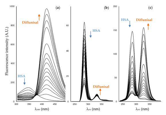
**Figure 2.** Fluorescence spectrum for diflunisal-HSA at: (a) Emission; (b) synchronous  $\Delta \lambda = 15$  nm; (c) synchronous  $\Delta \lambda = 60$  nm modes. The sixteen additions of diflunisal performed to cover the ratio 0.7:13 with respect to the initial concentration of HSA in the cell (4.5  $\mu$ M).
