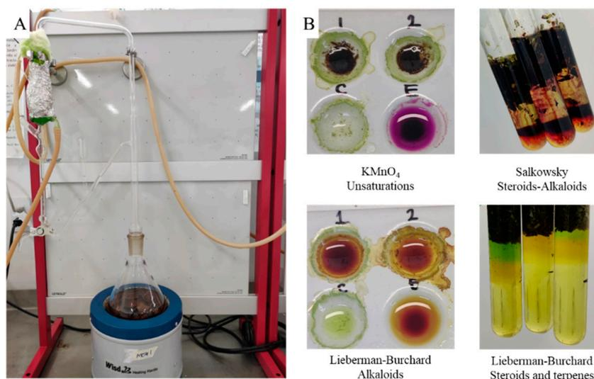
**Figure 2.** (A) The modified Cleverger extraction system. (B) Representative phytochemical tests from fresh plant material.
