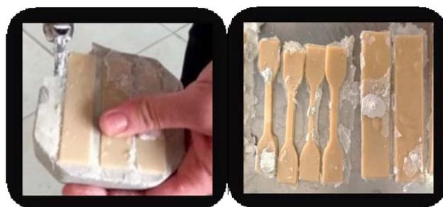
**Figure 3.** Divesting resin samples.
