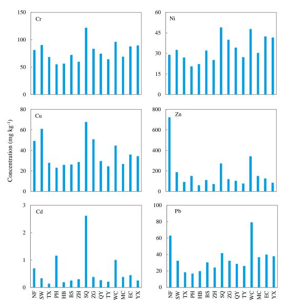
**Figure 2.** Cr, Ni, Cu, Zn, Cd, and Pb concentrations in sediments from 15 sampling sites. Specifically, there are 11 samples (NF, SW, TX, PH, HB, BS, ZH, SQ, ZG, QY, and TY) corresponding to 11 rivers flowing into Lake Chaohu, 3 samples (WC, MC, and EC) from Chaohu, and 1 sample (YX) from the river flowing out of Chaohu.
