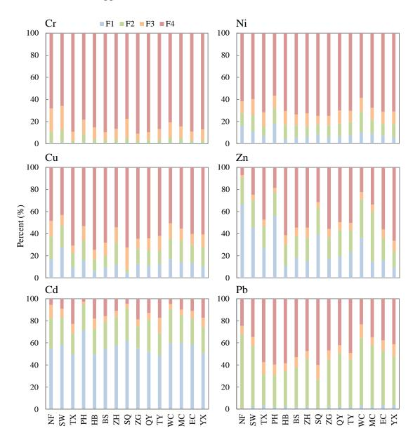
**Figure 5.** Percentages of Cr, Ni, Cu, Zn, Cd, and Pb existing as different fractions of the BCR sequential extraction procedure for sediments sampled at 15 sites. F1, exchangeable and carbonate included fraction; F2, reducible fraction; F3, oxidizable fraction; and F4, residual fraction.
