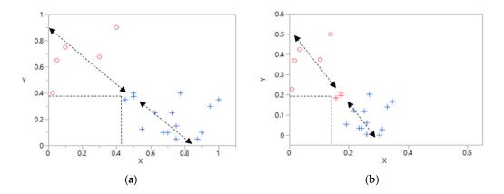
Figure B1. (a) Clustering in the original coordinate system; (b) Clustering using scaled coordinates.
