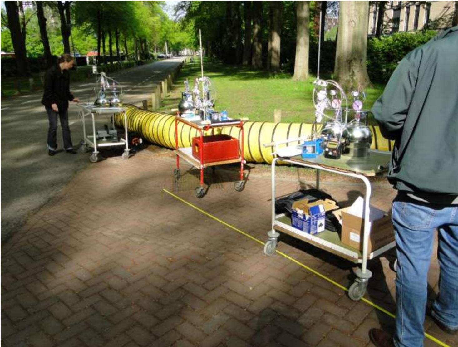
Figure S2: Set-up for emission measurements at the emission point of the power supply (end of yellow tube). The photograph was taken before the engine was started.
