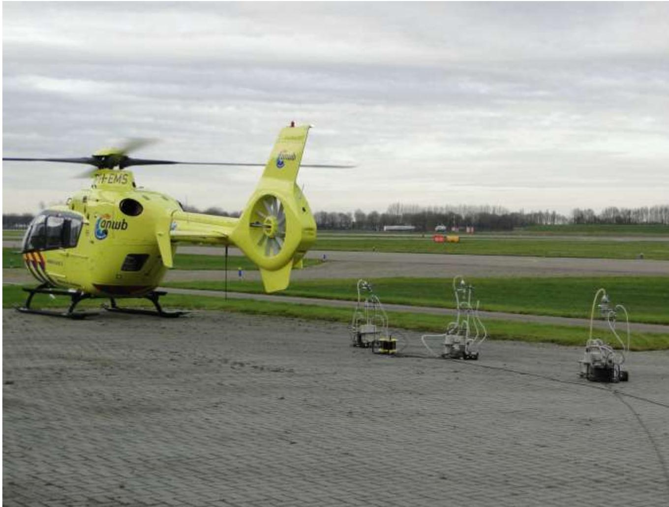
Figure S1: Helicopter emission measurement at the airport in Lelystad.
