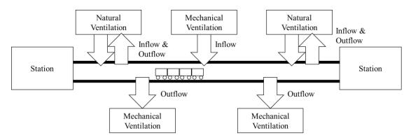
Figure 1. The natural and mechanical ventilation systems in line 4.
