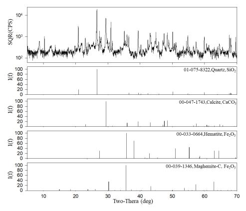
Figure 8. X-ray diffraction (XRD) patterns of PM in the subway tunnel at the S station.
