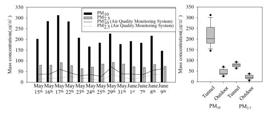
Figure 4. Particulate matter (PM) mass concentration in the subway tunnel at the M station.
