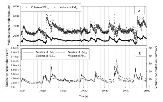
**Figure 5.** The number and volume of PM in the subway tunnel at the M station between 7:00 and 8:00 p.m. on 15 May 2017.
