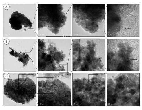
Figure 13. Morphology of PM in subway tunnels according to size at the S station.
