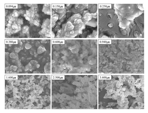
Figure 11. Morphology of PM in subway tunnels according to size at the M station.
