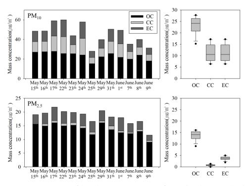
Figure 7. Mass concentrations of the carbonaceous components of PM in the subway tunnel at the M station (*n* = 13). OC—organic carbon; CC—carbonate carbon; EC—elemental carbon.
