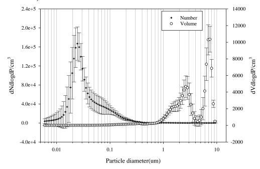
**Figure 6.** Size distribution of PM in the subway tunnel at the M station between 7:00 and 8:00 p.m. on 15 May 2017.
