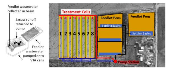
**Figure 1.** Vegetative Treatment System (VTS) design at beef cattle feedlot site. Feedlot runoff from pens is collected in settling basins, than routed to the pump station, and pumped onto treatment cells consisting of cool season grasses.
