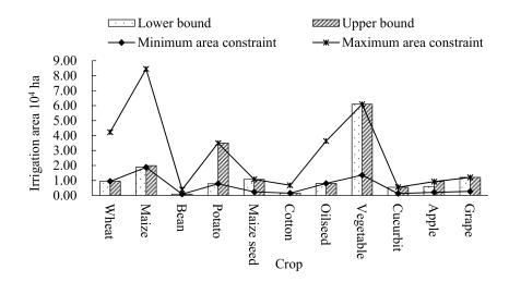
**Figure 7.** Optimal allocation area distribution for 11 crops ( $\lambda i = 30\%$ ,  $P_i = 0.1$ ) and the maximum and minimum crop area constraints.
