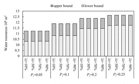
**Figure 8.** Irrigation water resources of different water-saving modes under different violation probabilities,  $P_{i}$ .
