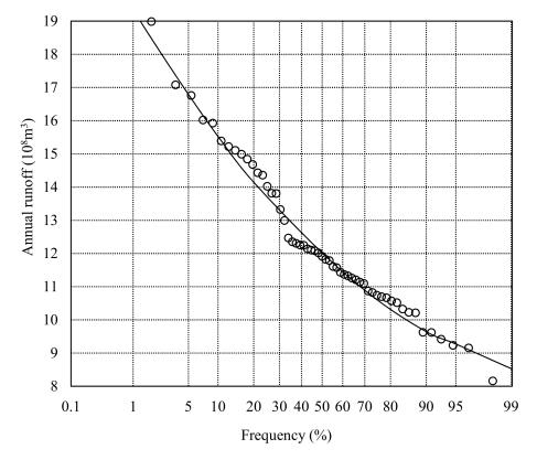
Figure 3. The P-III hydrographic curve.
