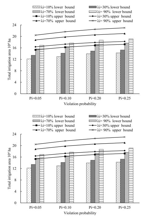
Figure 4. The total irrigation area of different water-saving modes under different violation probabilities, P<sub>i</sub>.
