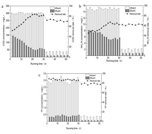
**Figure 4.** Chart of chemical oxygen demand (COD) (**a**), ammonia nitrogen (NH<sub>3</sub>-N) (**b**), and total phosphorus (TP) (**c**) removal during the start-up stage.
