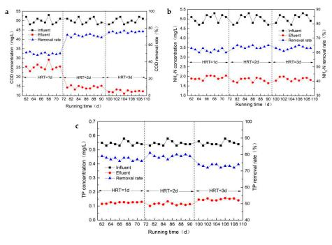
**Figure 5.** Chart of COD (**a**), NH<sub>3</sub>-N (**b**), and TP (**c**) removal under different hydraulic retention times (HRTs).
