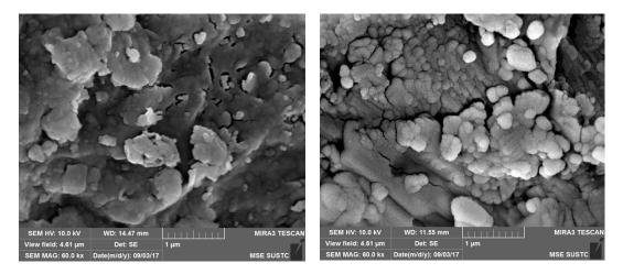
Figure 2. SEM images of the sludge ceramsite before (left) and after (right) it was roasted.
