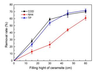
Figure 6. Chart of COD, NH<sub>3</sub>-N and TP removal at different filling heights.
