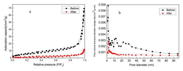
Figure 3. Nitrogen adsorption-desorption isotherms (a) and pore size distribution (b) of ceramsite.
