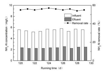
Figure 7. Chart of NH<sub>3</sub>-N removal when the influent NH<sub>3</sub>-N exceeded the standard.
