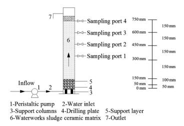
Figure 1. Schematic diagram of the experimental device for the constructed wetland.
