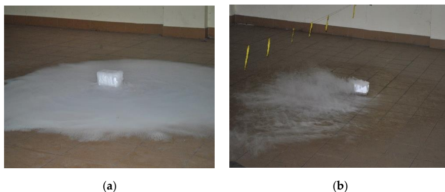
Figure 7. The dry ice test results: (a) jet fan ventilation system turned off; (b) jet fan ventilation system activated.
