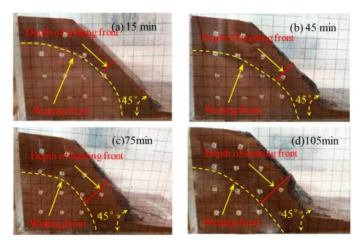
**Figure 4.** The characteristics of the 45° slope wetting front in rainfall conditions: (**a**) 15 min, (**b**) 45 min, (**c**) 75 min, and (**d**) 105 min.
