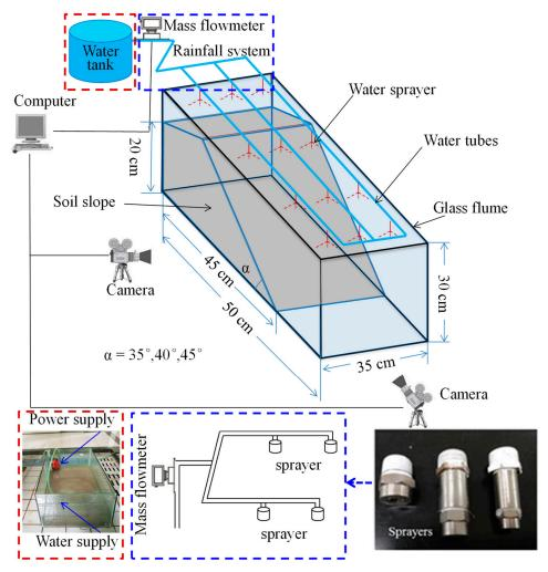
Figure 1. The schematic diagram of slope rainfall failure test device (SRFTD).
