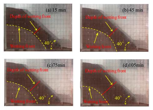
**Figure 3.** The characteristics of the 40° slope wetting front in rainfall conditions: (**a**) 15 min, (**b**) 45 min, (**c**) 75 min, and (**d**) 105 min.
