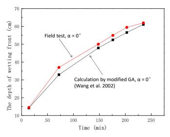
**Figure 10.** Comparison of calculation and field test values of wetting peak depth ( $\alpha = 0^{\circ}$ ).
