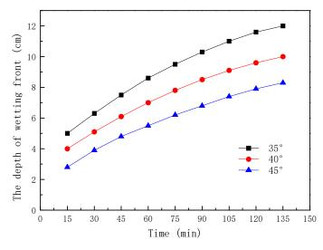
Figure 5. The depth of the wetting front with different slopes.
