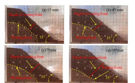
**Figure 2.** The characteristics of the 35° slope wetting front in rainfall conditions: (**a**) 15 min, (**b**) 45 min, (**c**) 75 min, and (**d**) 105 min.
