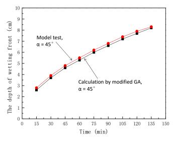
**Figure 9.** Comparison of calculation and model test values of wetting peak depth ( $\alpha = 45^{\circ}$ ).
