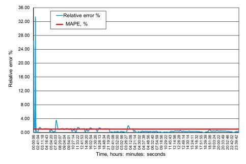
**Figure 14.** Percentage relative errors and mean forecasts of methane concentration levels in the MRW-3 measurement point.
