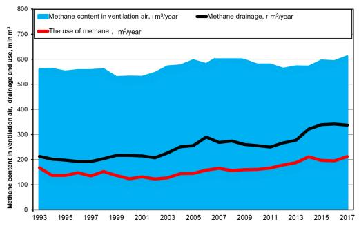
Figure 1. The amount of methane released into the atmosphere in Polish hard coal mines.
