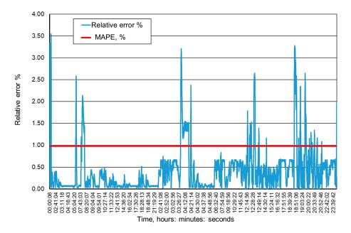
**Figure 15.** Percentage relative errors and mean forecasts of methane concentration levels in the MRW-4 measurement point.
