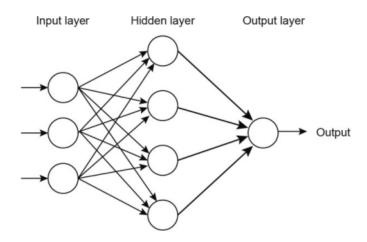
**Figure 6.** Typical Multilayer Perceptron (MLP) feed-forward Artificial Neutral Network Structure modified from [49].
