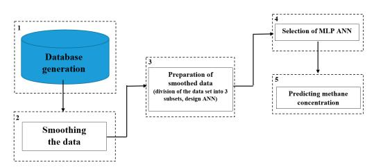
Figure 8. Methodological steps necessary to realize performing methane concentration.
