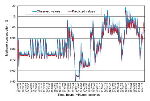
**Figure 12.** The time course of the registered and predicted methane concentration levels in the MRW-4 measurement point.
