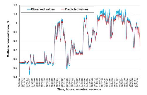
**Figure 9.** The time course of the registered and predicted methane concentration levels in the MRW-2 measurement point.
