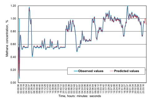
**Figure 10.** The time course of the registered and predicted methane concentration levels in the MRW-3 measurement point.
