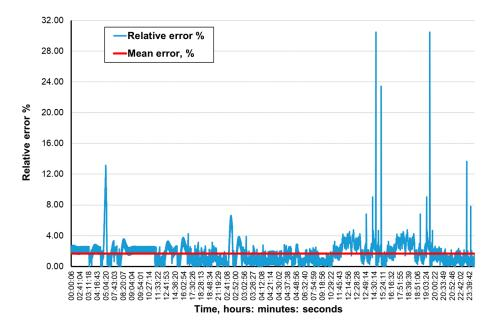
**Figure 13.** Percentage relative errors and mean forecasts of methane concentration levels in the MRW-2 measurement point.
