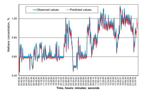
**Figure 11.** The time course of the registered and predicted methane concentration levels in the MRW-4 measurement point.
