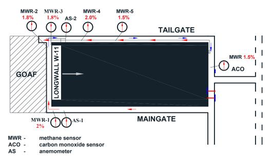
Figure 4. The distribution of sensors for measuring air parameters in the region of the longwall examined.
