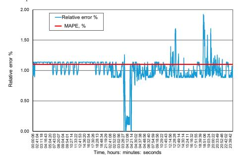
**Figure 16.** Percentage relative errors and mean forecasts of methane concentration levels in the MRW-5 measurement point.
