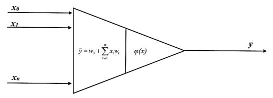
Figure 5. The basic model of a neuron, modified from [29].
