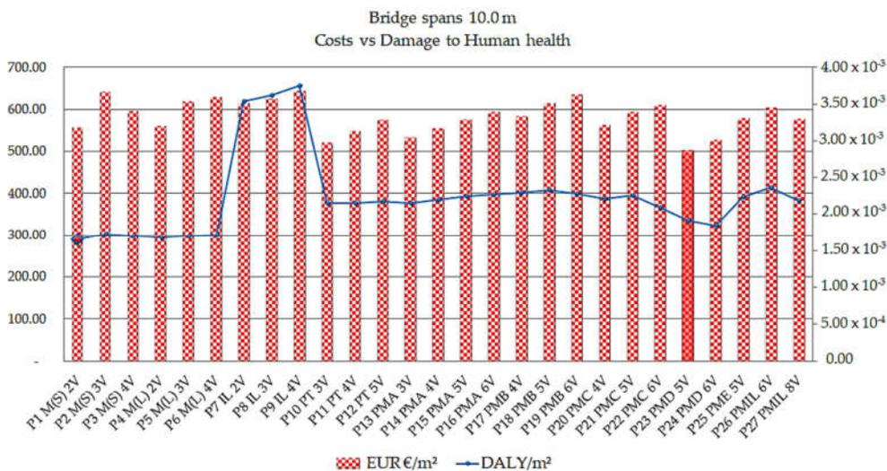
Figure 13. Cost times human health damage indices in EUR/m² and DALY/m² for the 10 m span.
