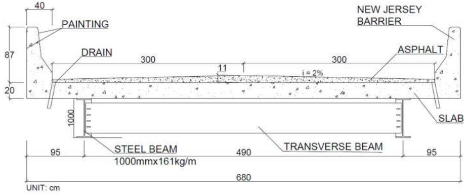
STEEL AND CONCRETE COMPOSITE BRIDGE 2 BEAMS
