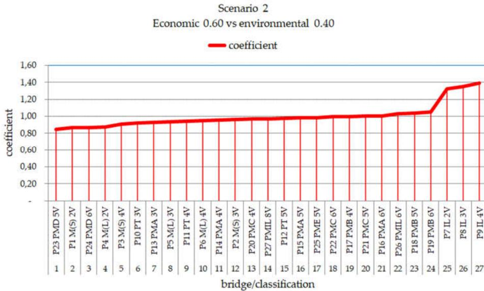
**Figure 15.** Classification of environmental performance with weights of 0.6 for economic and 0.4 for environmental factors per m<sup>2</sup> for bridges with lengths of 10 m.
