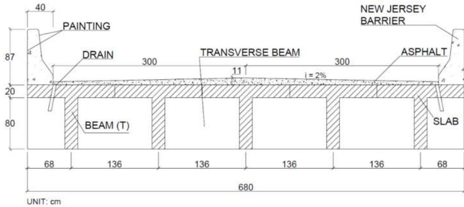
Precast concrete bridge - 5 beams
