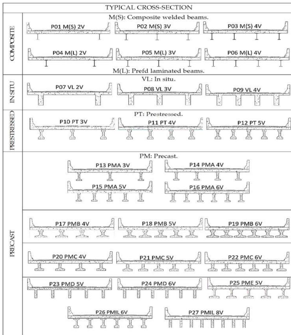
**Figure 1.** Number of bridges assessed: 27 typologies, 405 total bridges ranging from 6 to 20 meters.
