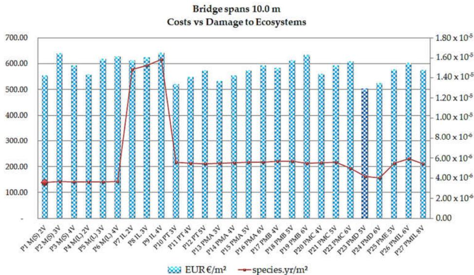
Figure 11. Cost x ecosystem damage indices in EUR/m<sup>2</sup> and species.yr/m<sup>2</sup> for the 10 m span.
