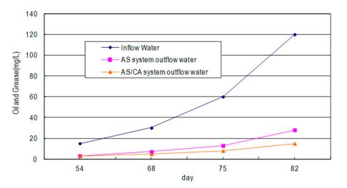
Figure 7. Treating oil and grease using AS system and AS/CA system.
