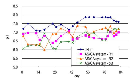
Figure 4. pH value of synthetic domestic sewage treated using AS/CA system.
