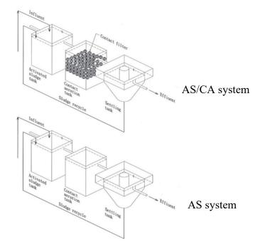
**Figure 1.** Flow chart of small model factory with activated sludge (AS) and activated sludge/contact aeration (AS/CA) systems.
