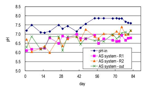
Figure 3. pH value of synthetic domestic sewage treated using AS system.
