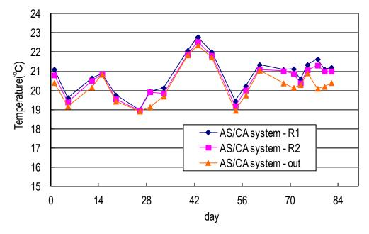
Figure 6. Temperature of synthetic domestic sewage treated using AS/CA system.
