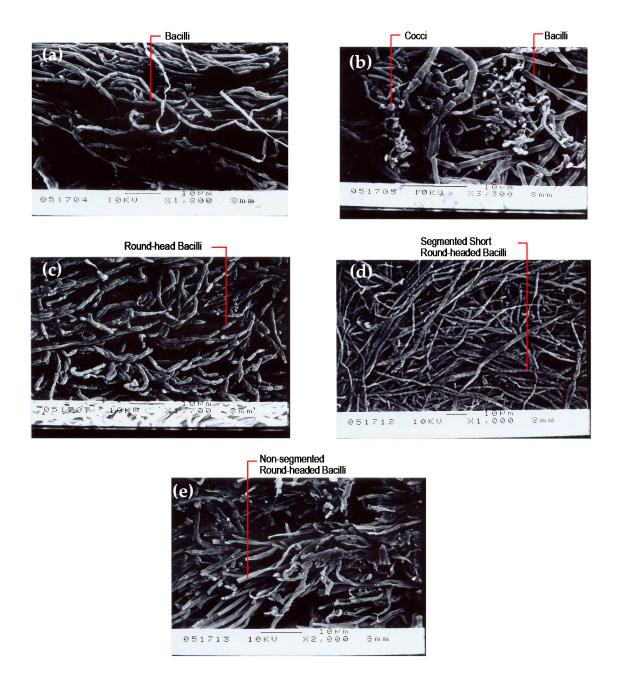
**Figure 8.** (a) Biological phase of first tank in AS system during stable period; (b) biological phase of second tank in AS system during stable period; (c) biological phase of first tank in AS/CA system during stable period; (d) suspended biological phase of second tank in AS/CA system during stable period; (e) fixed biological phase of second tank in AS/CA system during stable period; (e) fixed biological phase of second tank in AS/CA system during stable period; (b) biological phase.
