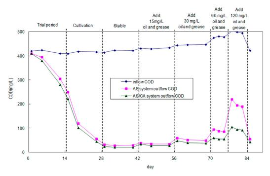
Figure 2. COD of synthetic domestic sewage treated by AS and AS/CA systems.
