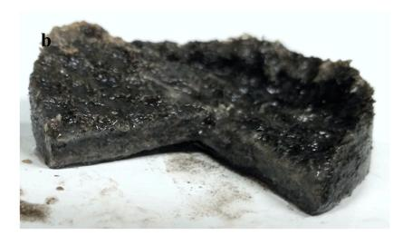
Figure 2. Photos of the clogging materials: (a) simulated gravel layer and (b) nonwoven geotextile layer.
