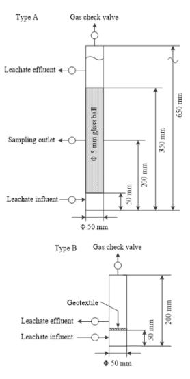
Figure 1. The schematic diagram of the simulation columns of leachate collection system (LCS).
