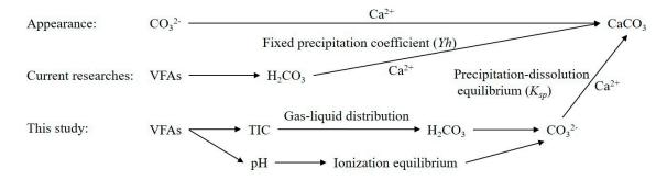
Figure 7. The calculating paths of biochemical reactions.
