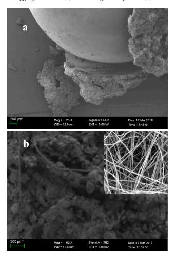
**Figure 3.** SEM pictures of the clogging materials: (**a**) the surface of glass spheres and (**b**) nonwoven geotextile fibers (upper-right corner is the SEM pictures of nonwoven geotextile before the experiment).
