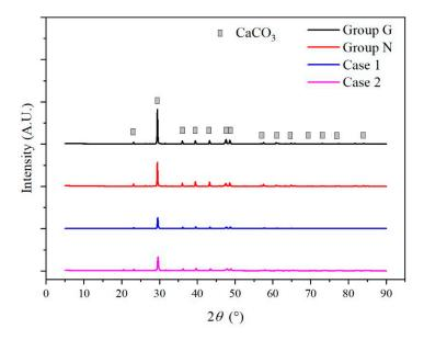
Figure 6. Crystal structure of the inorganic precipitates.
