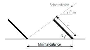
Figure 1. Diagram to calculate the minimum distance between collectors on a flat surface.
