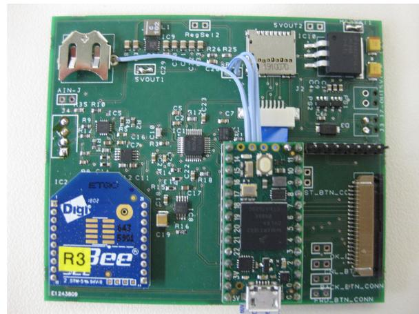
**Figure 3.** The main printed circuit board including the core elements of the HiFUSPEX prototype. Overall dimensions of the board: 85.2 mm × 72.5 mm.
