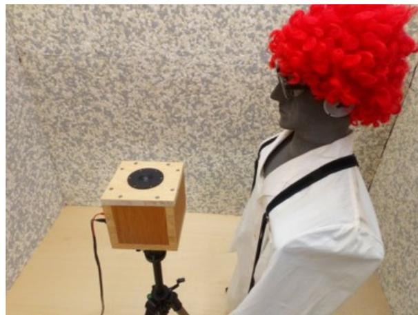
**Figure 5.** Experimental setup used for the simulation of an idealized sound field produced by an ultrasonic cleaning bath and a compressed air gun built within the free-field environment at the PTB Braunschweig, Germany.
