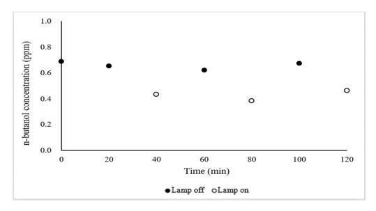
**Figure 6.** Mitigation of butan-1-ol (a.k.a. n-butanol) concentration with 110 UV-A lamps in the two chambers (#2 and #3). The reduction was measured by adding UV-A lamps inside two chambers. Black means light off, and white means light on. Airflow =  $0.25 \text{ m}^3/\text{s}$ , inlet air temperature =  $13 \degree \text{C}$ , outlet air temperature =  $19 \degree \text{C}$ , RH = 36% (inside mobile laboratory).
