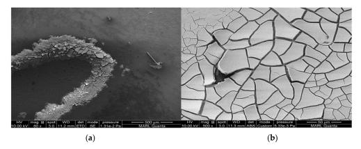
**Figure 7.** Sprayed TiO<sub>2</sub> coating arrangement in the 'valley' formed between the embossed fiberglass reinforced plastic (FRP). (a): 500  $\mu$ m & (b): 50  $\mu$ m magnification.
