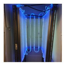
**Figure A4.** Picture of additional portable UV-A lamps installed inside Chamber #2 to densify light intensity.
