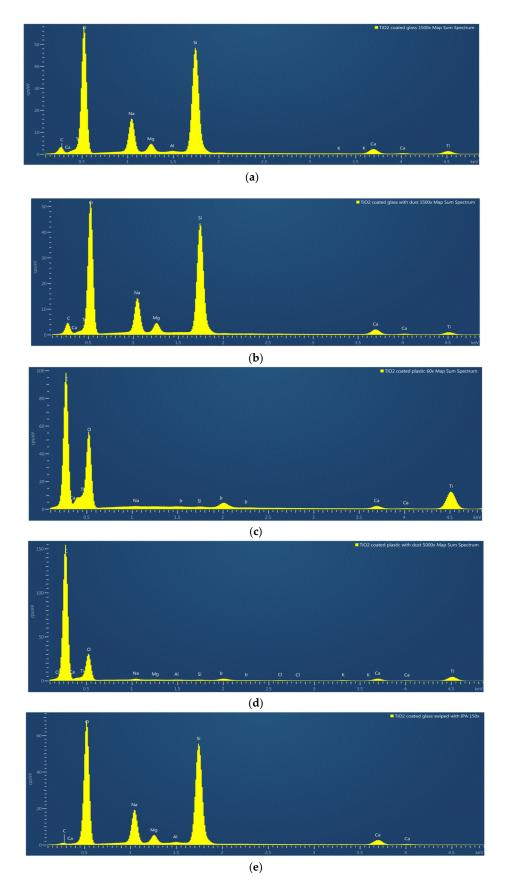
**Figure A9.** Chemical components detected on surfaces of common building materials. (**a**): glass, (**b**): glass with poultry dust, (**c**) The 'valley' part of the embossed fiberglass reinforced plastic (FRP) surface, (**d**): The embossed part of FRP with accumulated poultry dust, (**e**): glass with propan-1-ol solvent (example of  $TiO_2$  removal from the surface).
