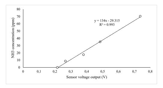
Figure 3. Calibration for real-time NH<sub>3</sub> measurements.
