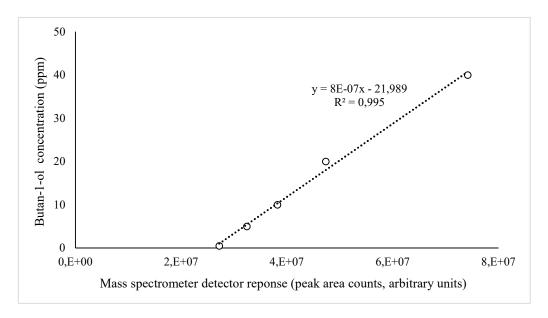
trometry (GC-MS) system for analyses (Agilent 6890 GC; Microanalytics, Round Rock, TX, USA). The calibration for butan-1-ol is shown in Figure 4.
