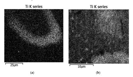
**Figure A8.** Map of  $TiO_2$  arrangement detected on the surface. White dots represent detected  $TiO_2$  coating. (a) glass surface, (b) fiberglass reinforced plastic (FRP) surface.
