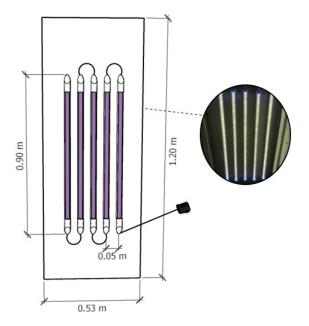
Figure A2. Schematic of UV-A lamps installation in the treatment chamber.
