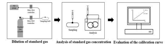
**Figure 2.** Calibration method for measuring targeted gas concentration. (1) Five standard gas concentrations were prepared/diluted to be within the range of the target gas to be measured. (2) Standard gas samples were analyzed with SPME-GC-MS or electrochemical gas sensors resulting in a gas concentration calibration curve.
