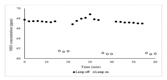
**Figure 5.** Mitigation of NH<sub>3</sub> concentration with 110 UV-A lamps inside the two chambers (#2 and #3, Figure 1). NH<sub>3</sub> concentration was measured at the effluent of chamber #3. Airflow =  $0.25 \text{ m}^3/\text{s}$ , inlet air temperature (influent of chamber #2) = 13 °C, outlet air temperature = 19 °C, RH = 36% (effluent of chamber #3). The y-axis start at 60 ppm (not 0).
