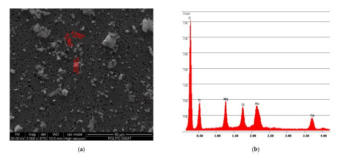
**Figure 20.** R airborne sample of abrasion simulation test with coarse-grained sandpaper. (**a**) SEM photo of Chrysotile free fiber bundle; (**b**) spectrum of Chrysotile with typical Mg and Si peaks.
