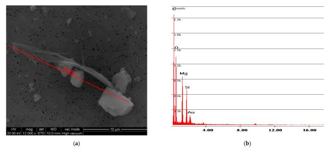
**Figure 19.** F airborne sample of abrasion simulation test with coarse-grained sandpaper. (a) SEM photo of Chrysotile bundle; (b) spectrum of Chrysotile with typical Mg and Si peaks.
