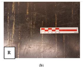
**Figure 3.** (a) Sample F—squared floor green tiles with white and black stripes, more flexible and in good condition (b) Sample R—squared floor black tiles with beige stripes, quite rigid and in fairly good condition.
