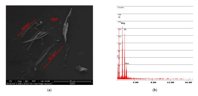
Figure 6. F sample SEM analysis. (a) Photo of free fibers of chrysotile with measurement values; (b) spectrum of chrysotile.
