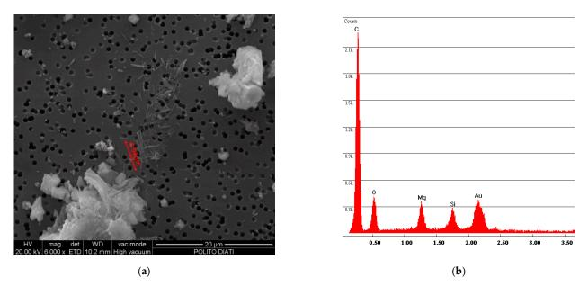
**Figure 18.** R airborne sample of abrasion simulation test with fine-grained sandpaper. (**a**) SEM photo of little Chrysotile free fibers;(**b**) spectrum of Chrysotile with typical Mg and Si peaks.
