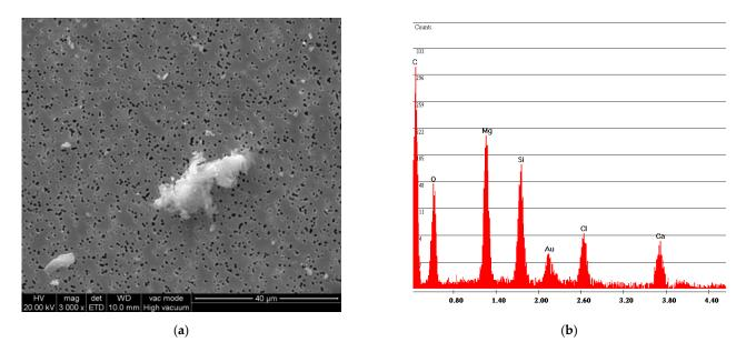
**Figure 15.** Sample R airborne sample of simulation for impact and drag with crampons. (**a**) SEM photo of incorporated asbestos fibers in the vinyl-adhesive matrix. (**b**) Spectrum with Mg and Si Chrysotile peaks and Cl and Ca adhesive matrix peaks.
