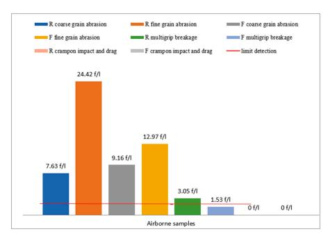
**Figure 21.** Histogram of the fiber/liter values calculated according to Ministerial Decree 06/09/1994 [4], for all tests carried out on samples R and F. The horizontal red line indicates the limit detection value.
