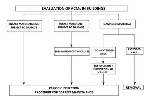
**Figure 2.** Evaluation scheme of asbestos-containing materials (ACMs) in building and recommendations (from Article 1, Annex: Standards and Technical Methods for Risk Assessment, Control, Maintenance and Remediation of Materials Containing Asbestos Present in Building Structure, Risk Assessment, Table 2 of M.D. 6/9/94 [4].
