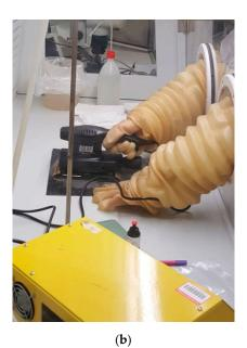
**Figure 11.** (a) Sandpaper used for the test. Left: fine sandpaper (dimensions: P120). Right: coarse sandpaper (dimensions: P40). (b) Performed mechanical abrasion test inside the confined hood.
