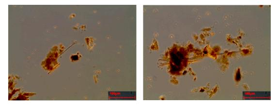
**Figure 12.** Phase-contrast microscope (PCOM) photos of the powder obtained by means of abrasion test. Chrysotile fiber with part of the vinyl glue remain attached.
