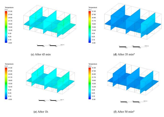
Figure 12. Temperature after the heating system was powered off; \* refers to heating without solar radiation.
