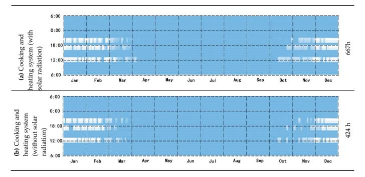
**Figure 13.** (**a**) Suitable time of the annual average for cooking and heating system with solar radiation; (**b**) Suitable time of the annual average for cooking and heating system without solar radiation.
