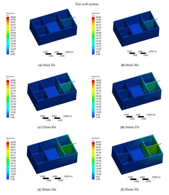
Figure 10. Wall heating for specific times.
