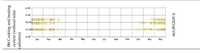
**Figure 14.** (**a**) The annual average load reduction in the cooking and heating system with solar radiation; (**b**) The annual average load reduction in the cooking and heating system without solar radiation.
