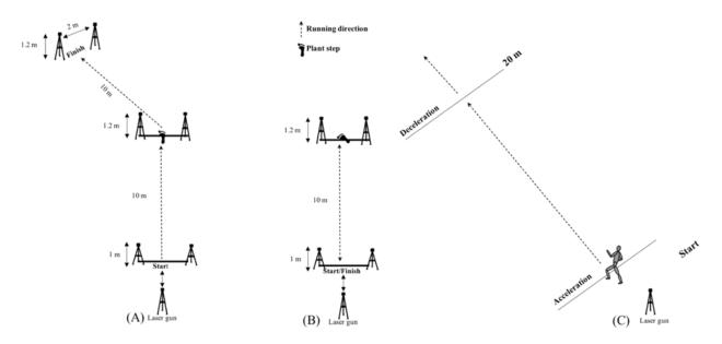
Figure 1. Set-up for maximum horizontal braking test (A), the 45° (B) and 180° (C) COD test.
