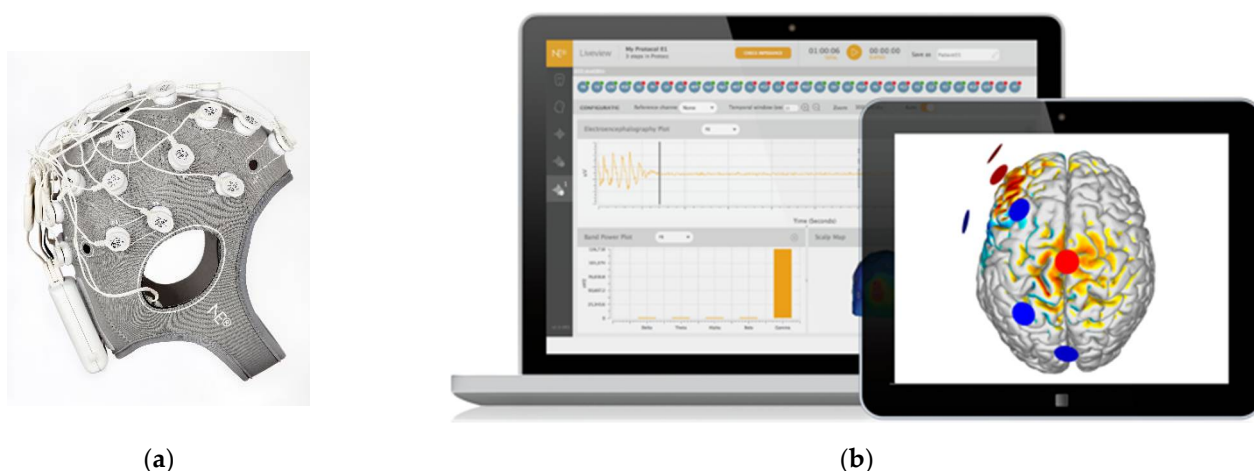
Figure 1. BRAINCODE's hardware and software: (a) medical certified EEG device ENOBIO; (b) NIC Desktop Software Platform (Software creator: Neuroelectrics, Barcelona, Spain. Version number: 2.1.0.).
