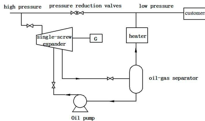
**Figure 1.** Schematic view of a basic high pressure natural gas pipeline with single-screw expander.
