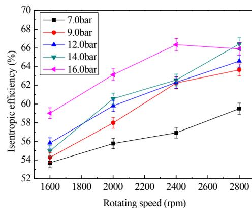
Figure 8. Isentropic efficiency versus rotating speed.
