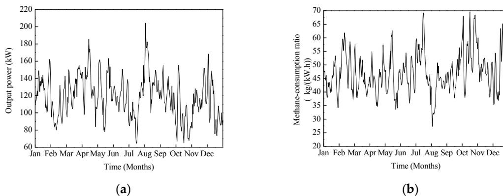
**Figure 13.** Predicted parametric curves of output power (a) and methane-consumption ratio (b).
