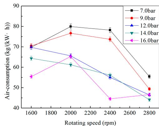
Figure 11. Air-consumption versus rotating speed.
