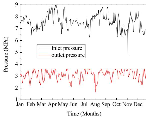
**Figure 12.** Inlet/outlet pressure of natural gas during 2014.
