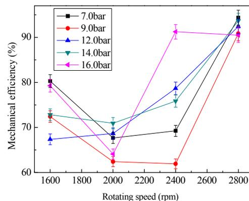
Figure 9. Mechanical efficiency versus rotating speed.
