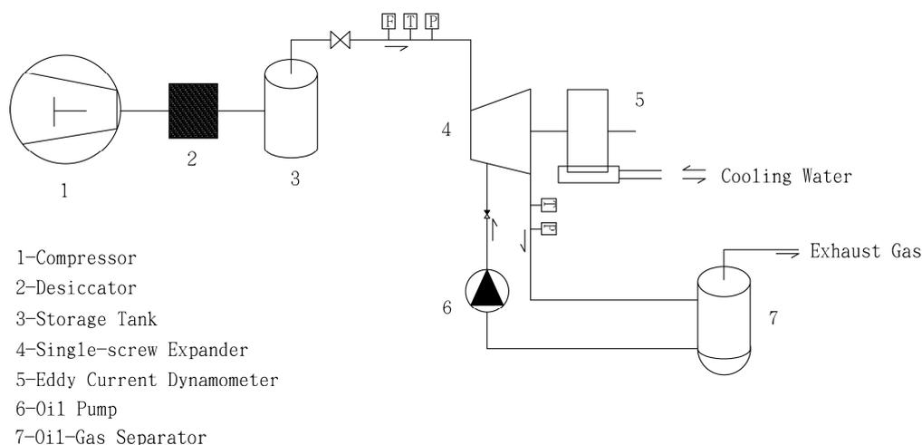
Figure 4. Schematic diagram of the experimental system.
