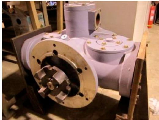
Figure 3. Photo of the single-screw expander prototype.
