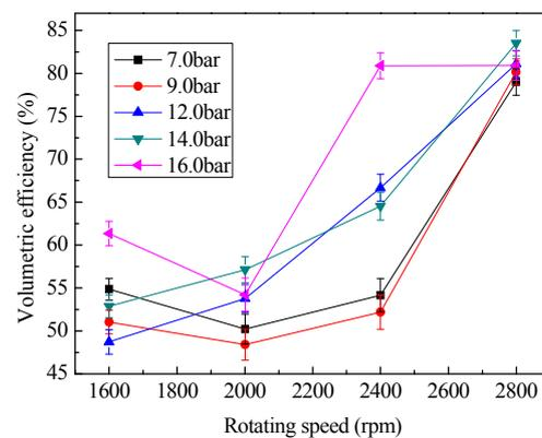
Figure 7. Volumetric efficiency versus rotating speed.
