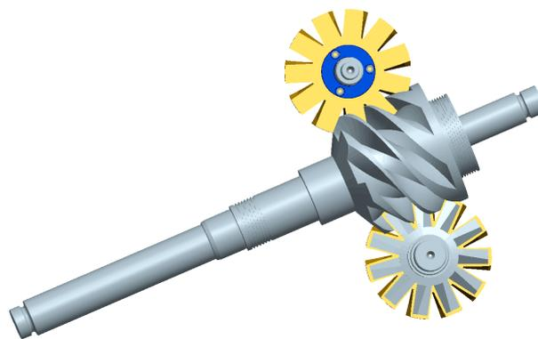
**Figure 2.** Three-dimensional structure of the single-screw expander.
