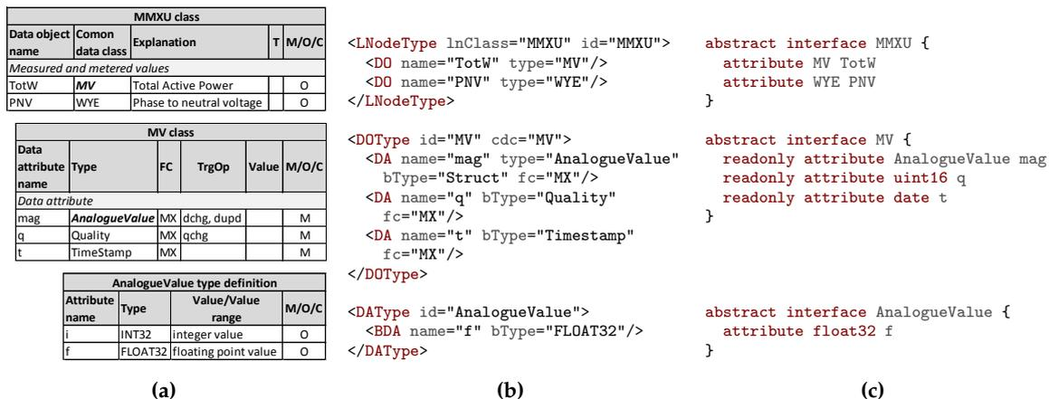
**Figure 9.** Mapping between an LN<sup>850</sup> and an <interface>: (a) Excerpt of the LN<sup>850</sup> MMXU in IEC 61850; (b) MMXU as SCL description; (c) MMXU as <interface> description.
