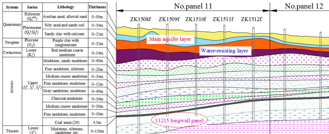
Figure 3. Stratigraphic column and section of No. 11 panel and No. 12 panel.
