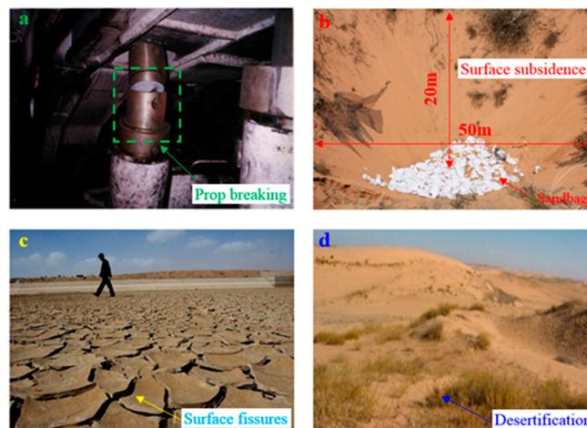
**Figure 1.** Geo-environmental hazards caused by coal mining. (a) Strong mining pressure; (b) Surface subsidence; (c) Soil and water loss; (d) Land desertification.
