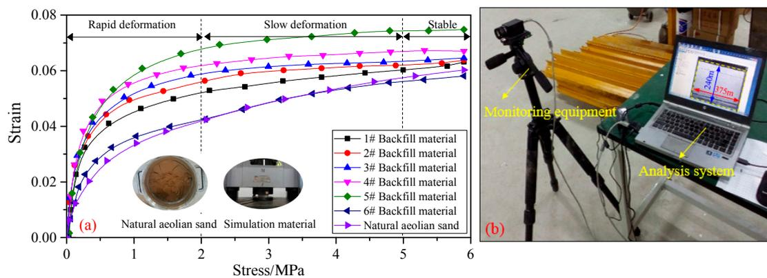
Figure 7. Physical simulation: (a) selection of similar backfill materials; (b) measurement system and software.
