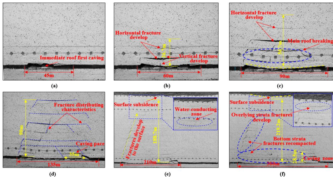
**Figure 9.** Development characteristics of overlying strata water-conducting fractures with caving method. (a) face advance of 45 m; (b) face advance of 60 m; (c) face advance of 90 m; (d) face advance of 135 m; (e) face advance of 210 m; (f) face advance of 300 m.
