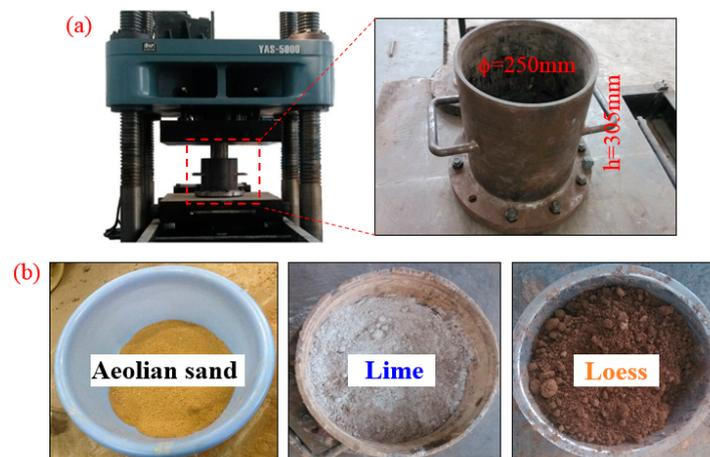
Figure 5. Experimental equipment and backfill materials. (a) Equipment; (b) Materials.
