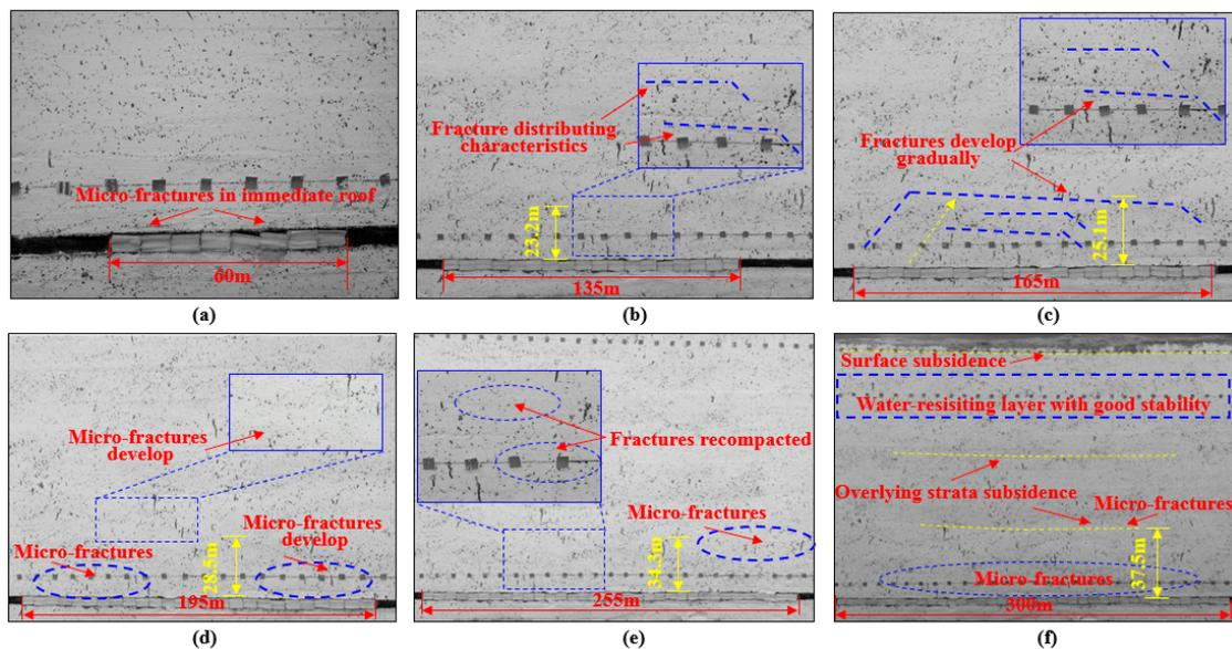
**Figure 11.** Development characteristics of overlying strata water-conducting fractures with BMCR of 90%. (a) face advance of 60 m; (b) face advance of 112.5 m; (c) face advance of 150 m; (d) face advance of 180 m; (e) face advance of 240 m; (f) face advance of 300 m.
