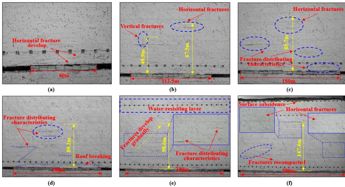
**Figure 10.** Development characteristics of overlying strata water-conducting fractures with BMCR of 70%. (a) face advance of 60 m; (b) face advance of 112.5 m; (c) face advance of 150 m; (d) face advance of 180 m; (e) face advance of 240 m; (f) face advance of 300 m.
