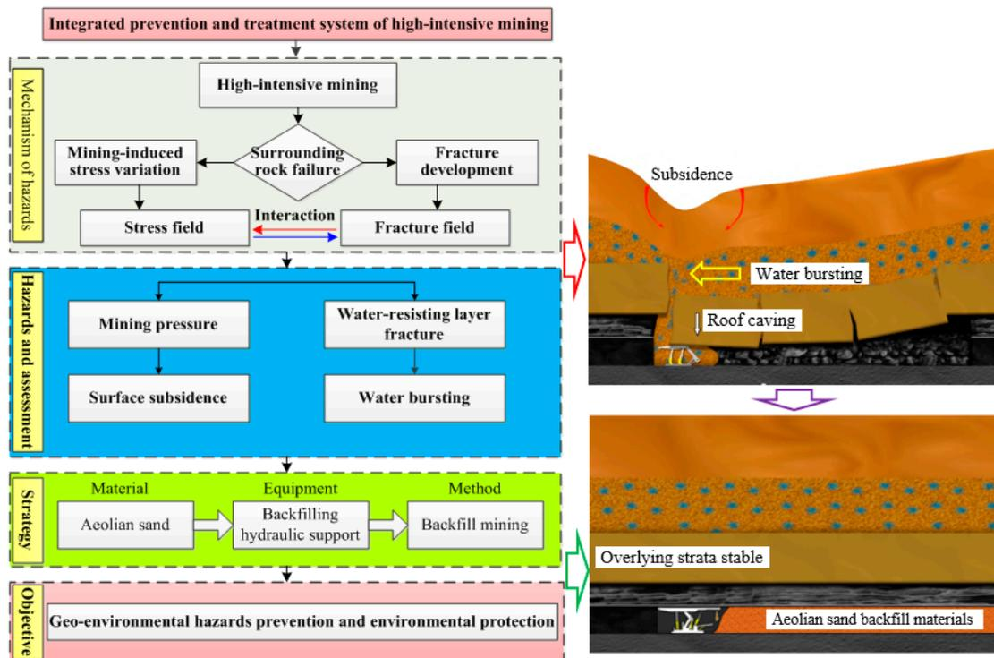
Figure 14. Integrated prevention and treatment system of high-intensive mining.
