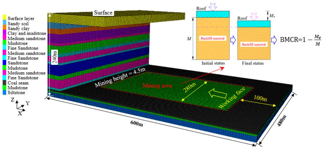
Figure 8. Sketch of the FLAC<sup>3D</sup> mesh for numerical simulation.
