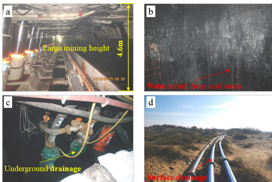
Figure 4. Water inrush and pumping-drainage system with high-intensive mining on site.
