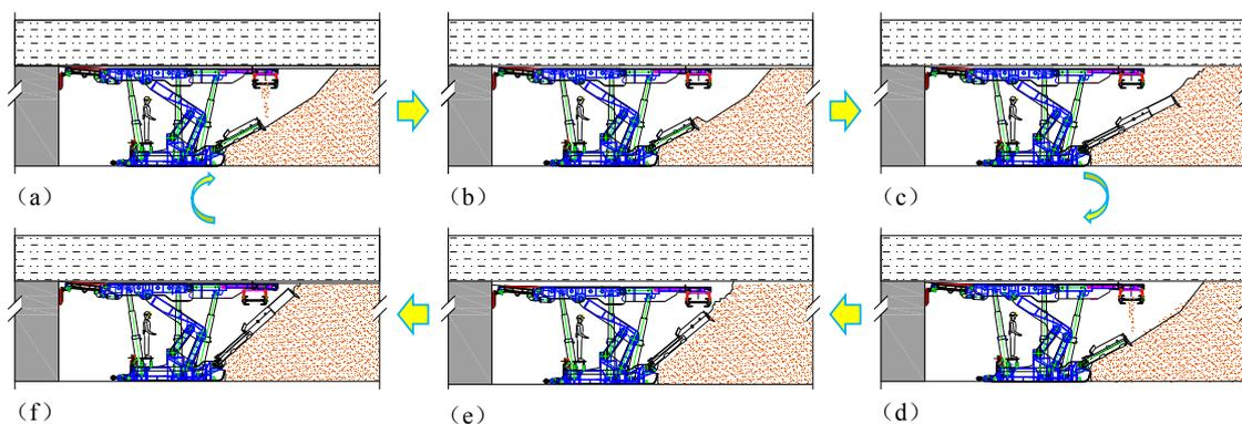
Figure 15. Technology and process of rapid-backfill coal mining with aeolian sand.
