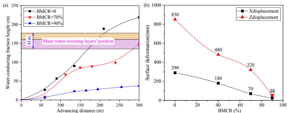
Figure 13. Fracture evolution and surface deformation with high-intensive mining.
