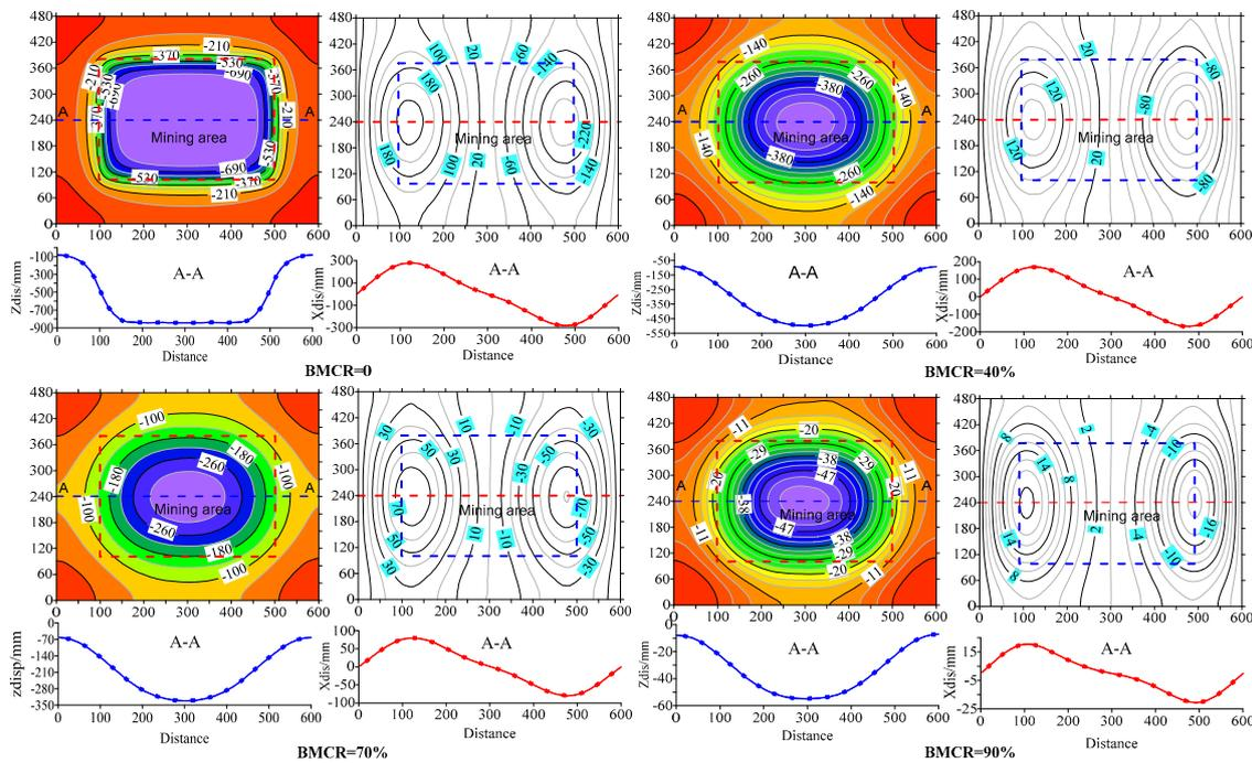
Figure 12. Development characteristics of surface deformation with BMCRs of 0, 40%, 70% and 90%.
