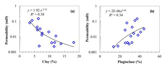
Figure 5. The cross plot of permeability with clay and plagioclase contents.
