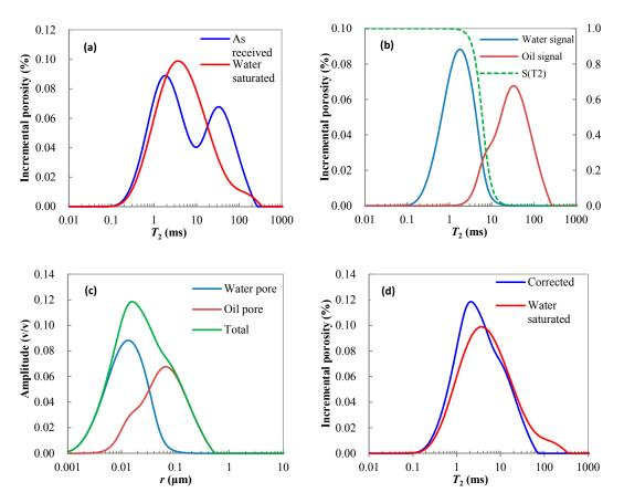
**Figure 7.** Sample M1: (a)  $T_2$  distributions for "as received" state and water saturated state; (b) Water and oil signal distributions obtained from "as received" state  $T_2$  distribution using weight function  $S(T_2)$ ; (c) Water-containing pore, oil-bearing pore and total pore size distributions; (d) Comparison of corrected and measured  $T_2$  distributions for water-saturated state.
