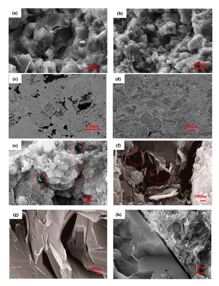
Figure 2. The pore types according to SEM analysis. (a) Intergranular dissolved pores; (b) Intergranular dissolved pores; (c) Intergranular and intragranular dissolved pores; (d) Intergranular and intragranular dissolved pores; (e) Illite/smectite mixed layer clay pores; (f) Chlorite clay pores; (g) Fracture pore; (h) Fracture pore.
