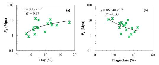
Figure 6. The cross plot of displacement pressure with clay and plagioclase contents.
