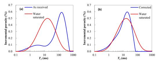
**Figure 8.** Sample M2: (a)  $T_2$  distributions for "as received" state and water saturated state; (b) Comparison of corrected and measured  $T_2$  distributions for water-saturated state.
