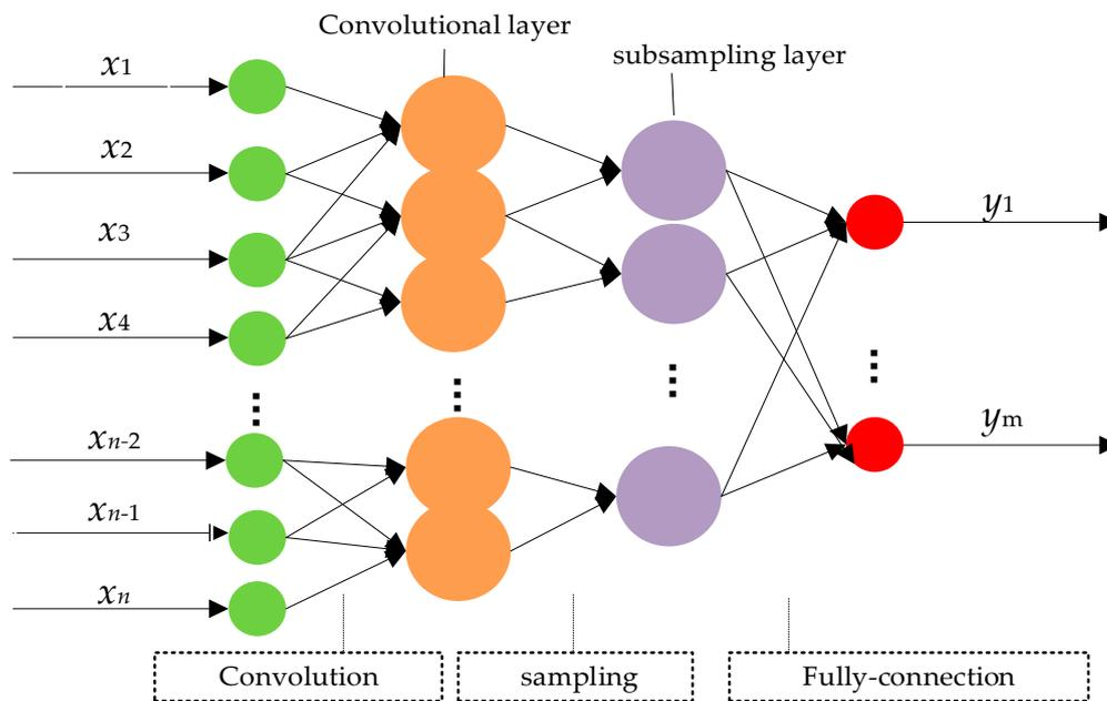
Figure 2. Convolutional neural network model.
