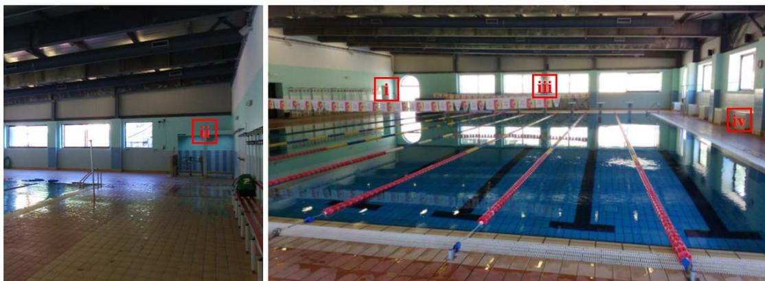
**Figure 7.** Locations of the air temperature and humidity sensors in the swimming pool hall: (i), edge of the swimming pool at a height of about 2 m; (ii) above the entrance of the dressing/bath zone; (iii) shorter wall of the swimming pool hall; (iv) one of the return air ventilation crates.
