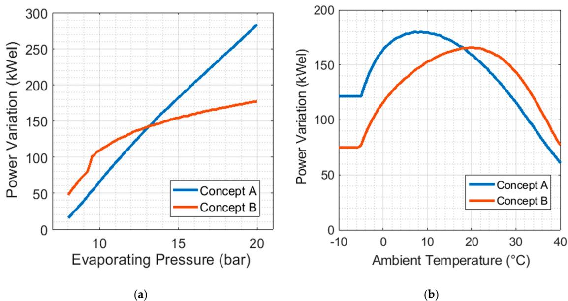
**Figure 4.** The difference between on- and off-design power is here represented for both concepts as a function of the evaporating pressure (a). Power variation is represented as a function of the ambient temperature (b).
