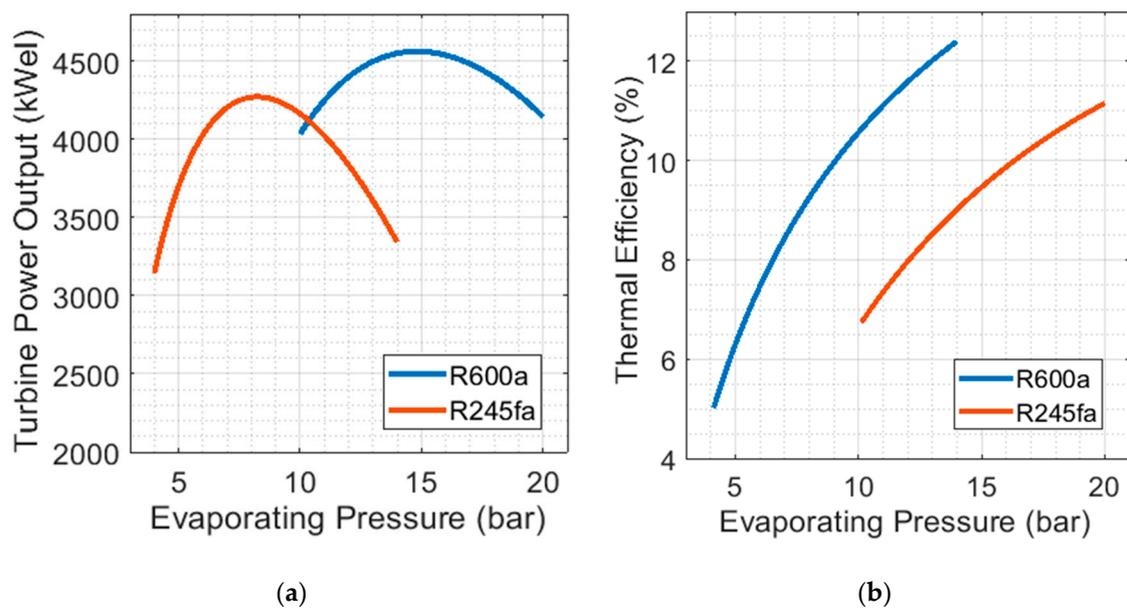
**Figure 3.** Turbine power is plotted as a function of the evaporating pressure, comparing R600a and R245fa as selected working fluid (a). Thermal efficiency is shown as a function of the evaporating pressure, comparing R600a and R245fa as selected working fluid (b).
