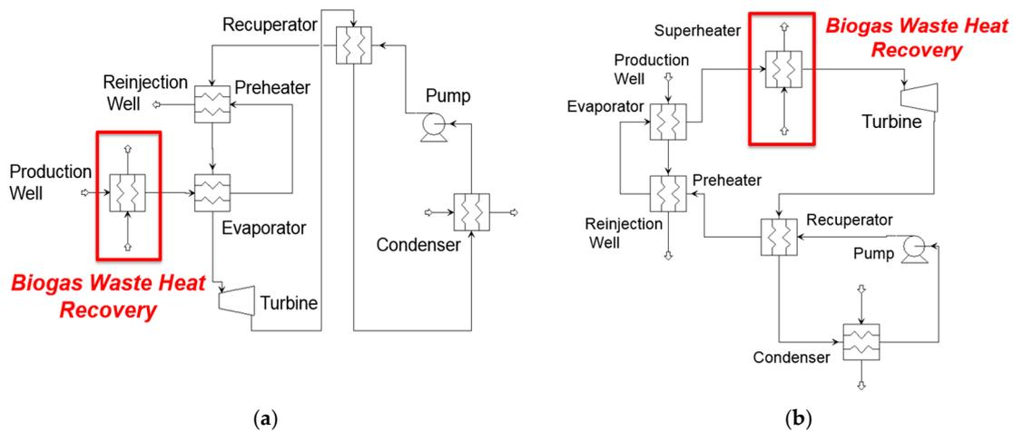
**Figure 1.** Concept A (a): Biogas waste heat is recovered preheating the geothermal water before entering the organic Rankine cycle (ORC) unit. Concept B (b): Biogas waste heat is exploited in order to superheat the working fluid before entering the turbine.
