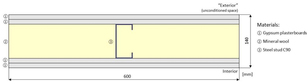
**Figure 2.** Cross-section of an interior LSF reference partition wall modeled on THERM software.
