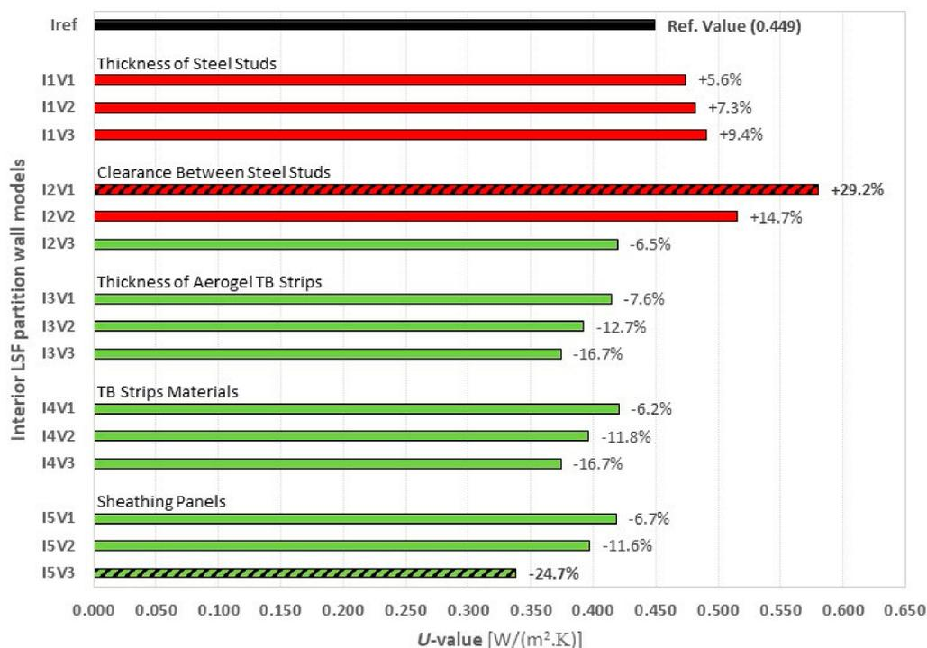
Figure 7. Thermal transmittances obtained for interior LSF partition walls.
