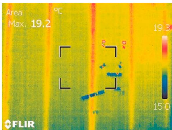
**Figure 1.** Thermal bridge's effect due to vertical steel studs in a light steel framed (LSF) wall captured in an infrared thermal image [30].
