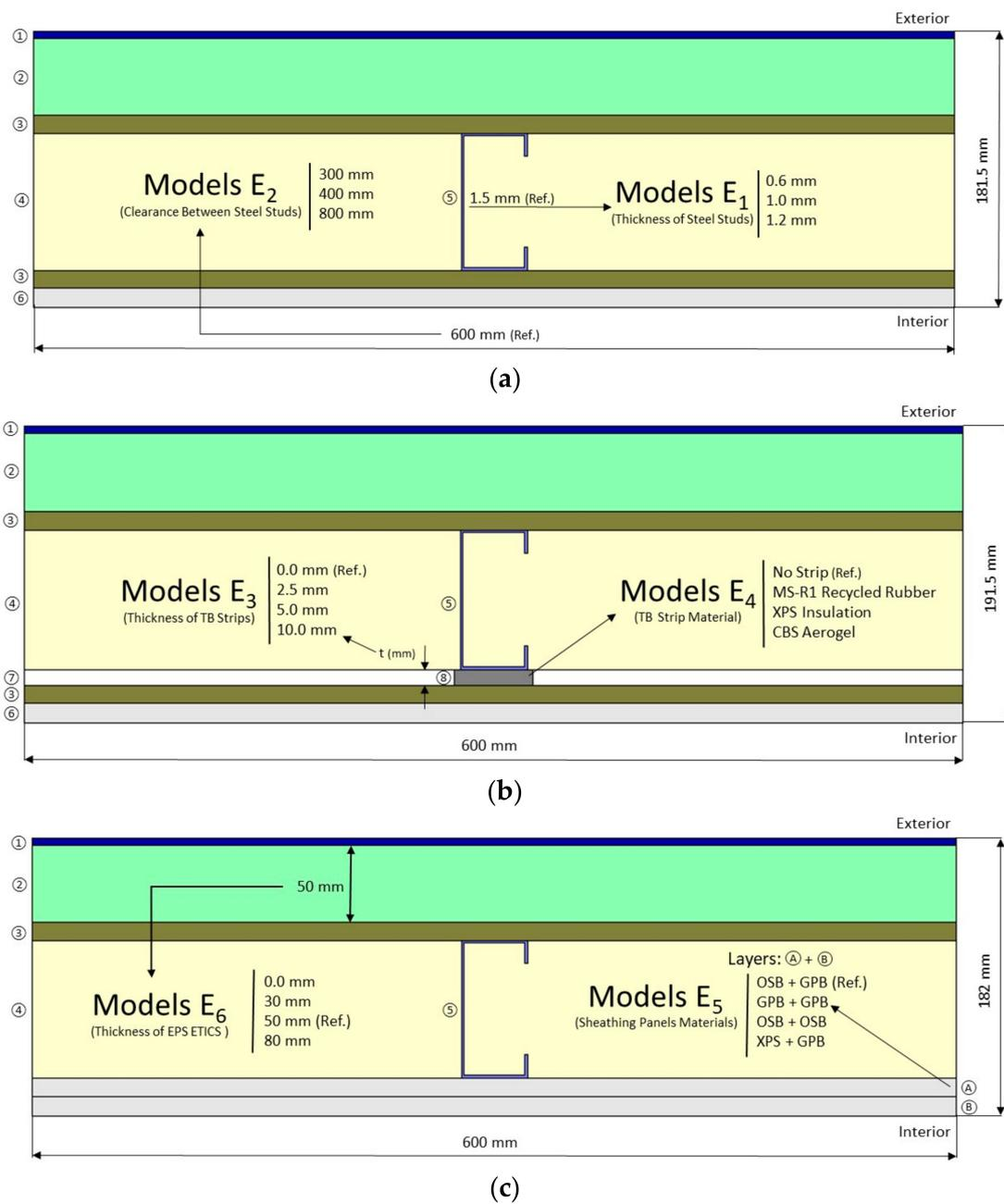
**Figure 5.** Exterior LSF facade cross-sections: (a) Models E1 and E2; (b) Models E3 and E4; (c) Models E5 and E6. Layers: ① ETICS finish; ② EPS; ③ OSB; ④ mineral wool; ⑤ steel stud C90; ⑥ gypsum plasterboard (GPB); ⑦ air layer; ⑧ TB strip.
