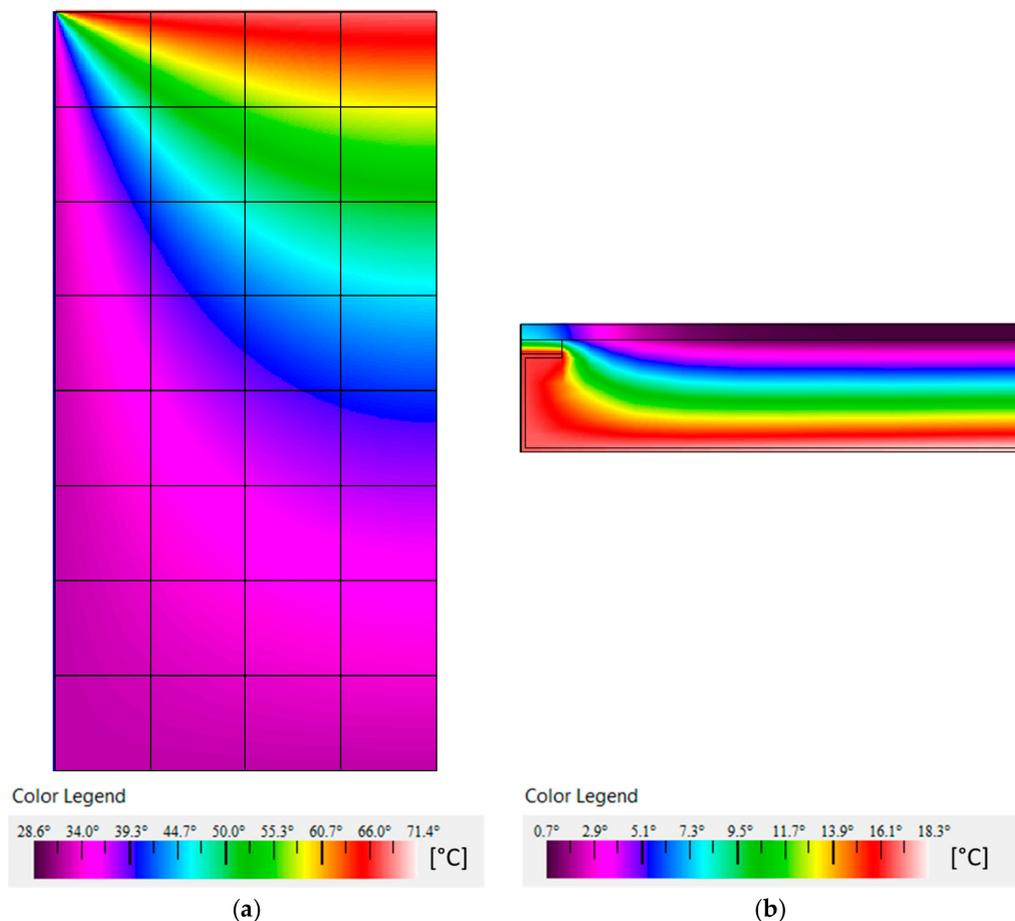
**Figure 6.** Temperature distribution obtained by the authors for the 2D test cases of ISO 10211 [22]: (a) test case 1; (b) test case 2.
