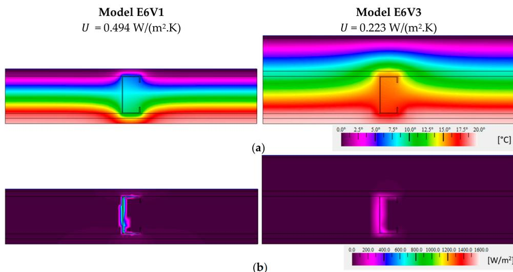
**Figure 10.** Temperature (a) and heat flux (b) color distribution for exterior LSF wall models with the highest  $U$ -value increase (0 mm EPS ETICS) and decrease (80 mm EPS ETICS).
