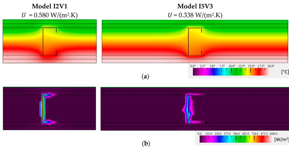
**Figure 8.** Temperature (a) and heat flux (b) color distribution for internal LSF wall models with the highest *U*-value increase (300 mm vertical stud distance) and decrease (XPS + GPB sheathing panels).
