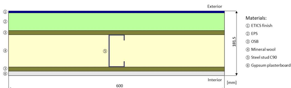
**Figure 4.** Cross-section of an exterior LSF reference wall modeled on THERM software.
