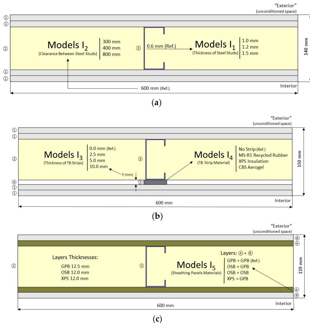
**Figure 3.** Interior LSF partition cross-sections: (a) Models I1 and I2; (b) Models I3 and I4; (c) Model I5. Layers: ① gypsum plasterboard (GPB); ② mineral wool; ③ steel stud C90; ④ air layer; ⑤ TB strip.
