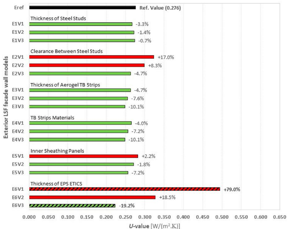
**Figure 9.** Thermal transmittances obtained for exterior LSF facade walls.
