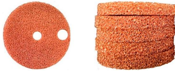
**Figure 7.** Porous medium: foam copper.
