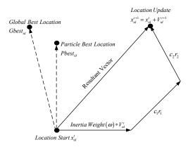
Figure 1. Particle swarm optimization (PSO) vector diagram.
