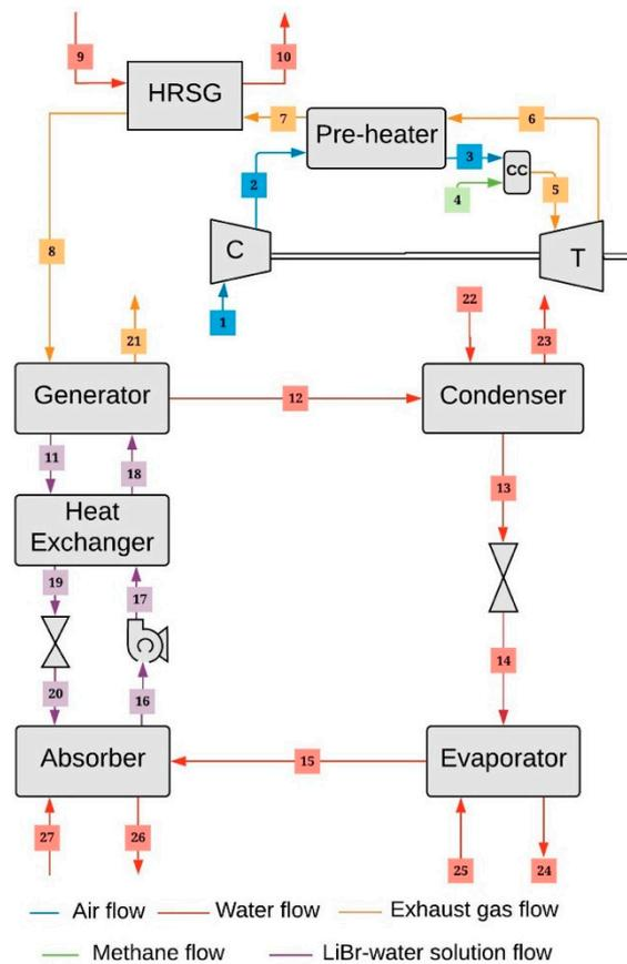
**Figure 1.** Physical structure of the trigeneration system.
